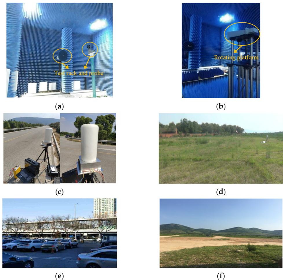
**Figure 2.** UCA radar data collection for different scenarios: (a) Microwave anechoic chamber test rack and probe; (b) Microwave anechoic chamber rotating platform; (c) Highway; (d) Dry grassland; (e) Town; (f) Gravel land.
