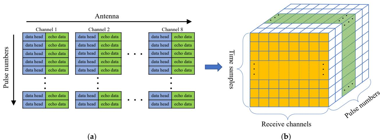
**Figure 3.** Radar data structure. (a) The storage format of echo data; (b) Radar data cube within a CPI.
