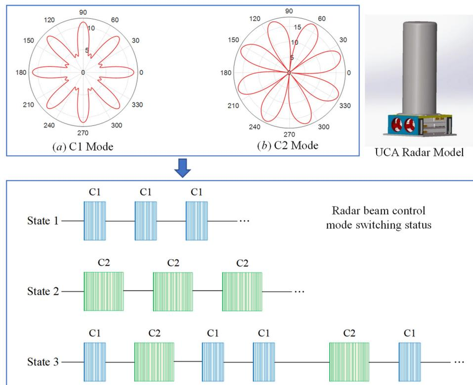
**Figure 1.** Switching states of two-beam control modes and corresponding beam pointing simulation pattern.
