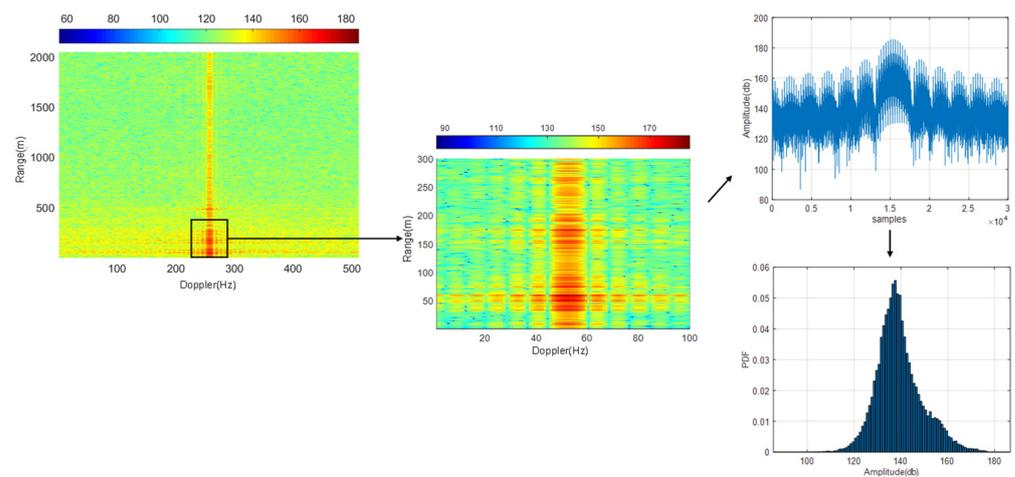
**Figure 6.** Schematic diagram of statistical parameter extraction of the range-Doppler map (Taking the dry grassland scene data as an example, 300 sample data are selected for the range unit, and 100 dimensions are chosen for the Doppler unit).
