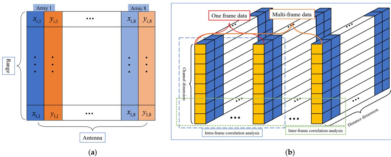
**Figure 5.** Schematic diagram of multi-dimensional data correlation analysis of UCA radar. (a) Schematic diagram of multi-channel single pulse data; (b) Schematic diagram of multi-channel and multi-pulse data.
