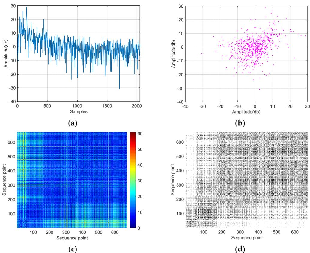
**Figure A2.** Recursive analysis results of range sampling signal of UCA radar ground clutter. The data comes from the UCA radar test experiment in the dry grassland scene. The scene's clutter background is relatively clean, and the change of the ground structure in each distance unit within the irradiation range of the beam in the fifth channel is noticeable. (a) One dimensional sampling signal in range direction; (b) Phase space plan; (c) State distance matrix; (d) Recursive plot.
