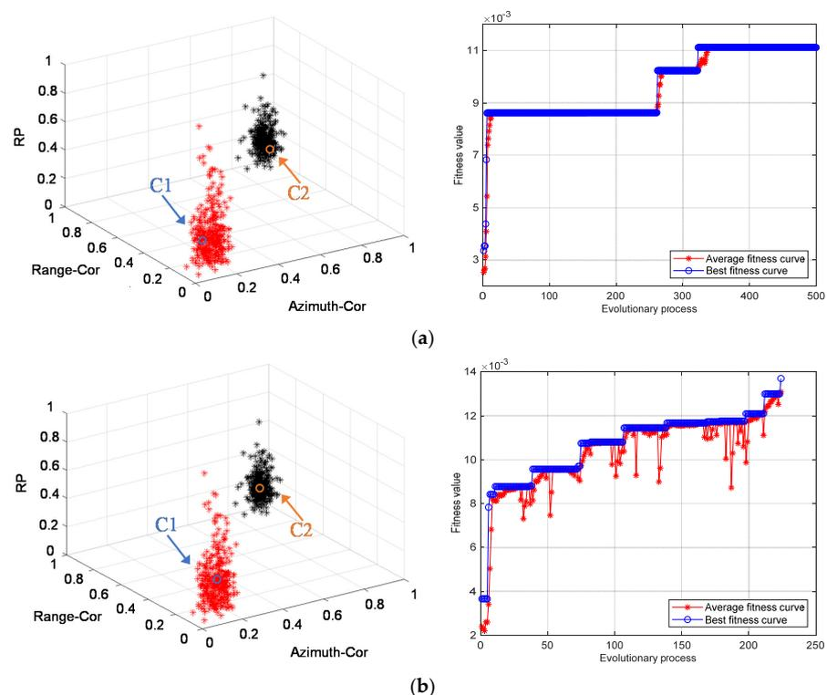
**Figure 9.** Clustering results of SGA (a) and chaotic SGA (b) in two-beam control modes. The population size is set to 15, and the maximum number of iterations is set to 500. The termination condition of the minimum criterion function value is 75. Note. The variables represented by the axis in the figure are dimensionless.
