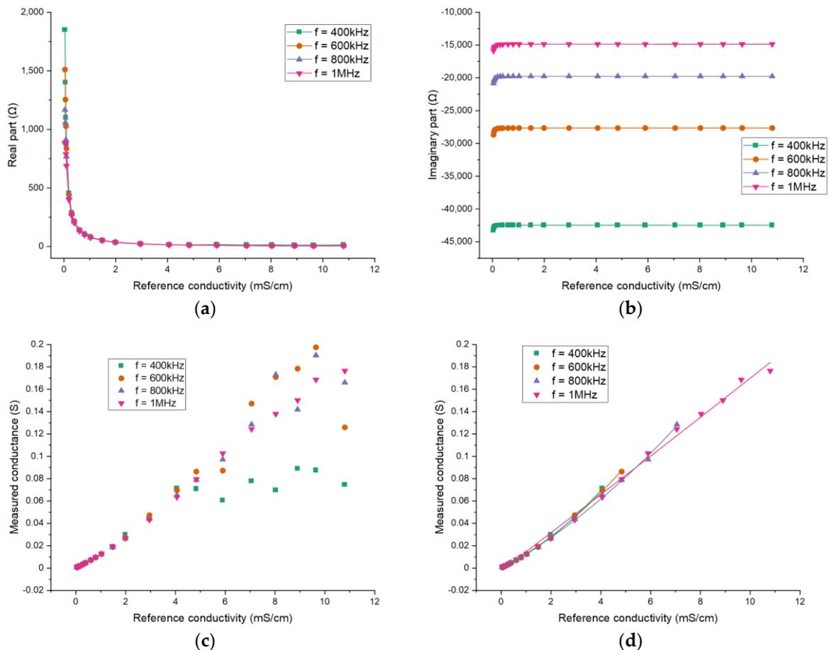
**Figure 12.** Experimental results for different excitation frequencies: The dependence of (a) the real part of the impedance; (b) the imaginary part of the impedance; (c) the measured conductance on the conductivity of the solution; (d) the conductance results with conductivity within the corresponding upper limit.
