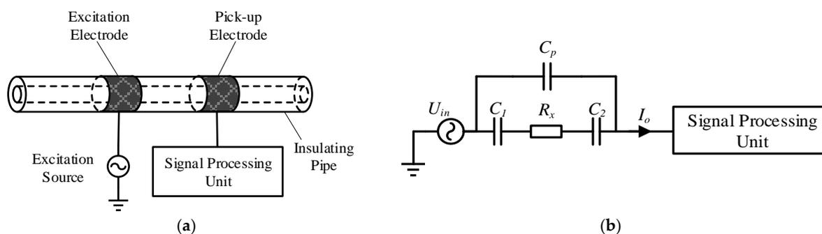
**Figure 1.**  $C^4D$  sensor: (a) The typical construction; (b) The equivalent circuit.
