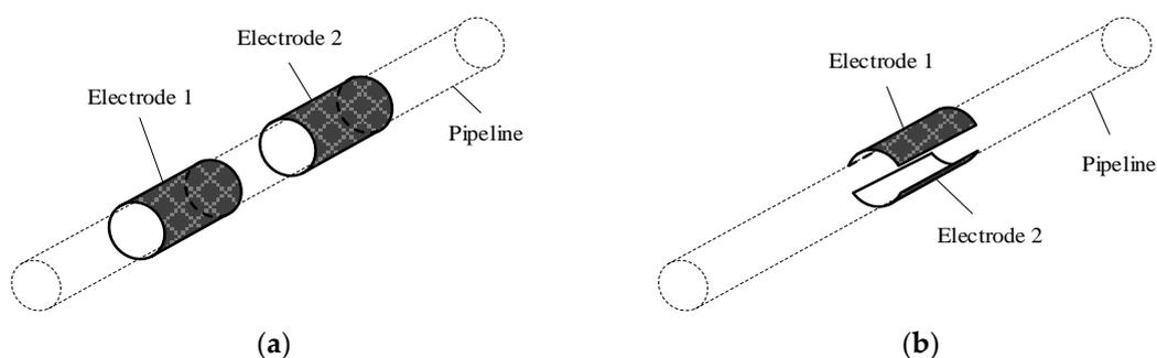
**Figure 2.** The  $C^4D$  sensor with different electrode configurations: (a) Tubular configuration; (b) Radial configuration. Notation: For the tubular configuration (as illustrated in (a)), a pair of cylindrical electrodes is attached around the pipe. For the radial configuration (as illustrated in (b)), a pair of concave electrodes is attached to the pipe oppositely.
