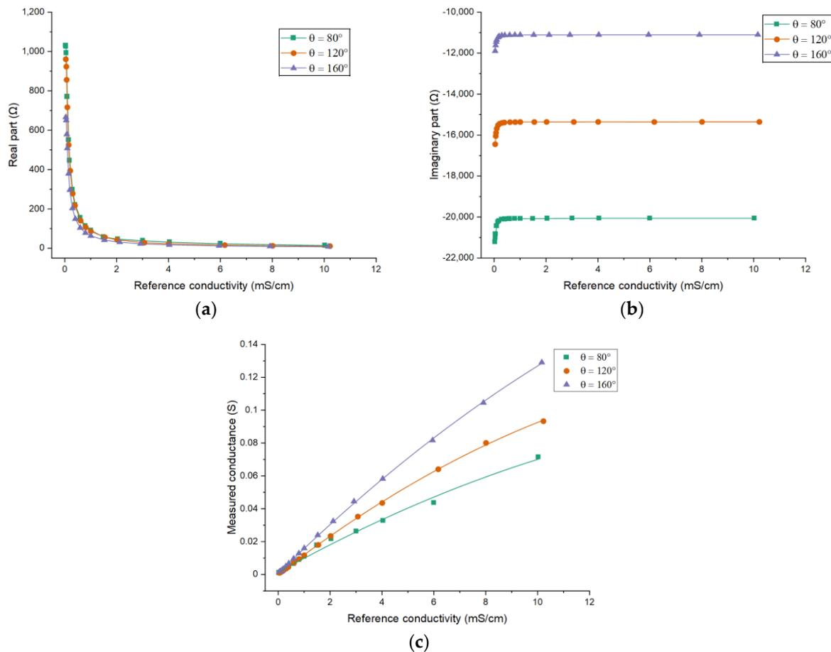
**Figure 14.** Experimental results for different electrode angles: The dependence of (a) the real part of the impedance; (b) the imaginary part of the impedance; (c) the measured conductance on the conductivity of the solution when  $L/d = 5.15$ .
