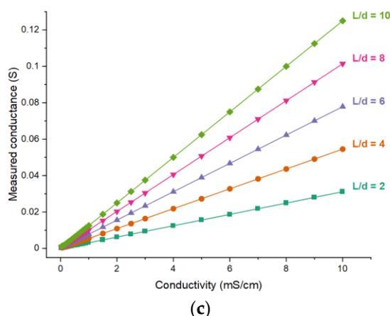
**Figure 9.** Simulation results for different electrode lengths: The dependence of (a) the real part of the impedance; (b) the imaginary part of the impedance; (c) the measured conductance on the conductivity of the solution when  $\theta = 120^\circ$ .
