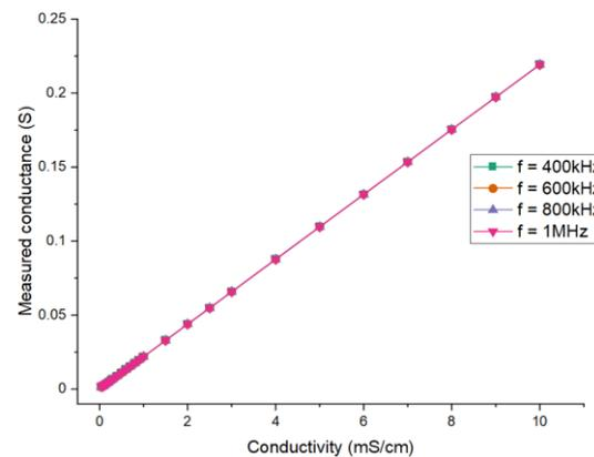
**Figure 8.** Simulation results for different excitation frequencies: the relationship between the measured conductance and the conductivity.
