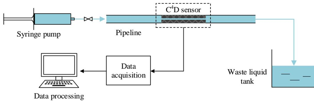
**Figure 11.** The layout of the experimental setup.
