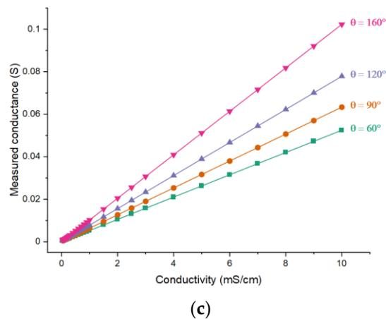
**Figure 10.** Simulation results for different electrode angles: The dependence of (a) the real part of the impedance; (b) the imaginary part of the impedance; (c) the measured conductance on the conductivity of the solution when  $L/d = 6$ .
