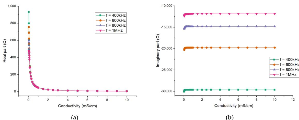
Figure 7. Simulation results for different excitation frequencies: The dependence of (a) the real part of the impedance; (b) the imaginary part of the impedance.
