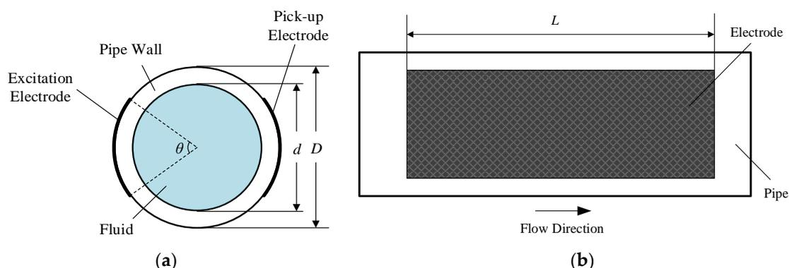
**Figure 3.** Views of the radial configuration: (a) The sectional view; (b) The lateral view.
