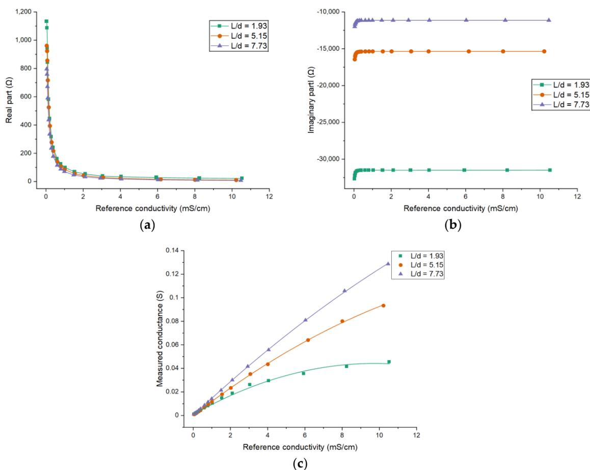
**Figure 13.** Experimental results for different electrode lengths: The dependence of (a) the real part of the impedance; (b) the imaginary part of the impedance; (c) the measured conductance on the conductivity of the solution when  $\theta = 120^\circ$ .
