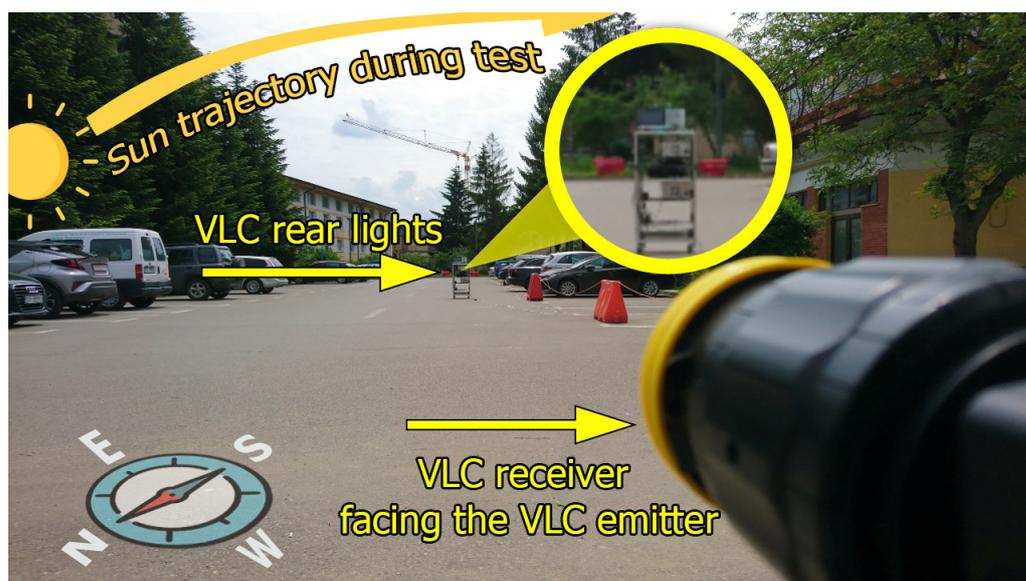
Figure 14. Outdoor experimental setup.
