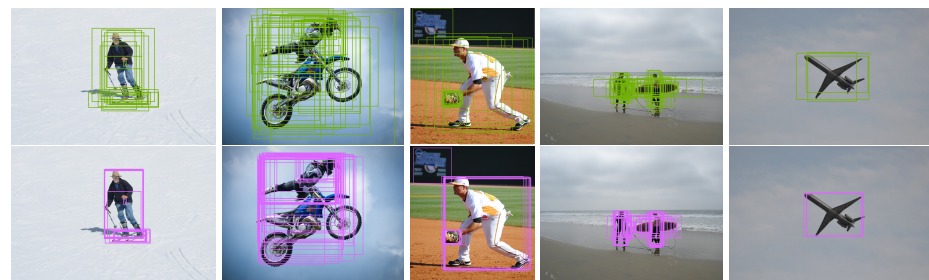
Figure 3. box_{rpn} (top) vs. box_{det} (bottom). The distributions of samples are intuitively different, and the regressed box_{det} have higher IoU with objects than box_{rpn} .
