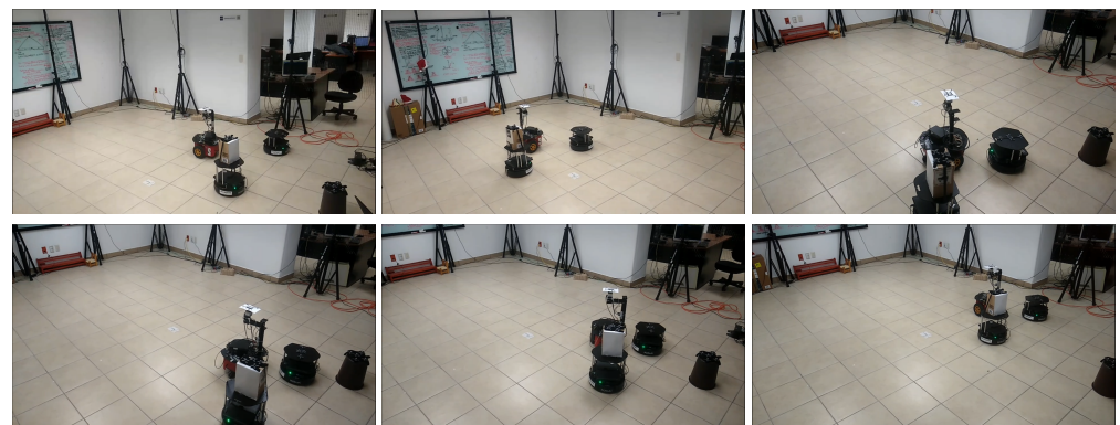
Figure 19. Three-agent system circular trajectory. Snapshots of the robots motion in the experiment. The initial configuration is at the top left and the final formation is at the bottom right. Intermediate positions when an obstacle is avoided are shown.
