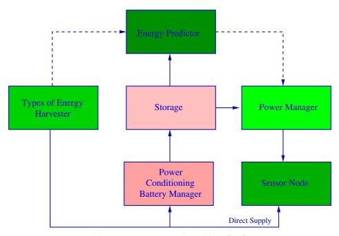
Figure 6. Components of a EH-WSN system. Adapted from [181].
