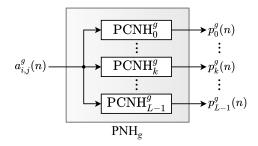
Figure 3. Architecture of the PNH<sub>g</sub>.
