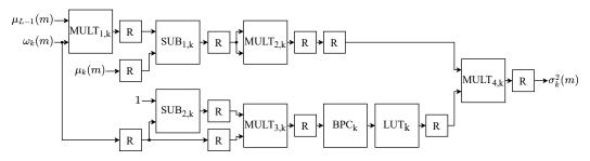
Figure 6. Architecture of the BCV<sub>k</sub> submodule.
