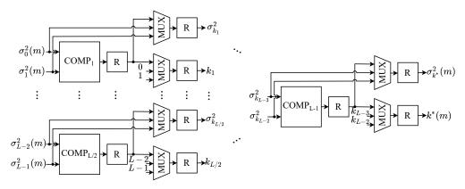
Figure 7. Architecture of the OTM.
