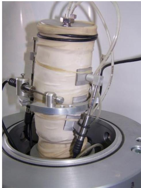
**Figure 5.** Sample of weak clay destroyed during the mounting of the sensors for strain measurement (source: photo of Jastrzębska M., after [41]; available via 2021 Civil and Environmental Engineering's permission).
