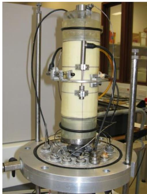
**Figure 3.** LVDT mounted on a sample (source: photo of Kowalska M., after [41]; available via 2021 Civil and Environmental Engineering's permission).
