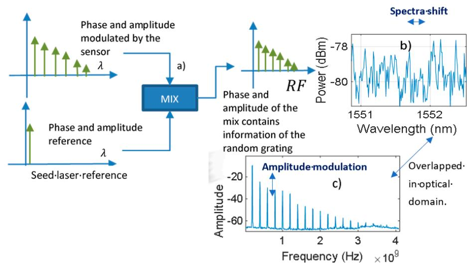
**Figure 1.** Demodulation: (a) mixing process that transduces the vibration measurement from the modulated optic spectra to RF; (b) optical reflection response of the random fiber sensor, which modifies the optical comb parameters; (c) spectra of the self-heterodyne comb.
