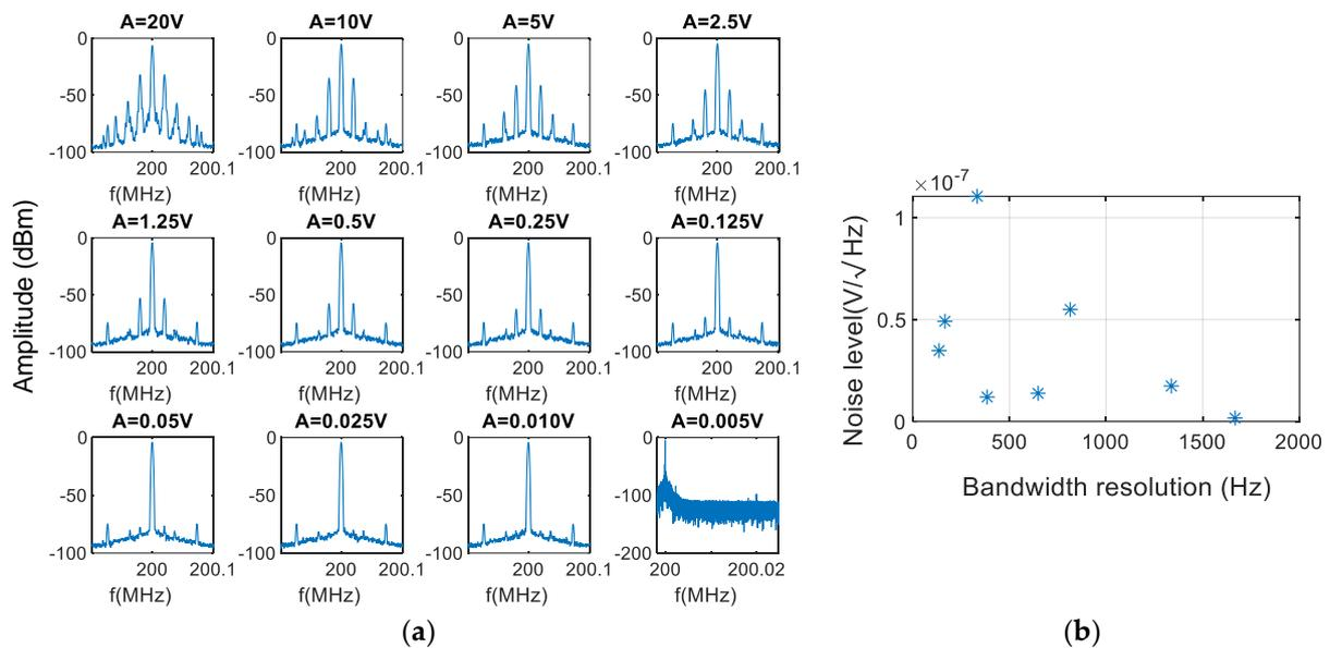
**Figure 4.** Calibrating interferometer: (a) response to different stimuli at 20 kHz generates a sideband modulation over the carrier. Ratios between the carrier and the first-order sidebands allow absolute calibration (A is the amplitude of the excitation voltage applied), (b) noise floor level achieved for different bandwidth resolutions.
