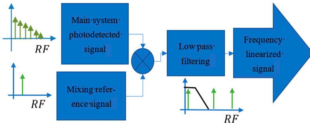
Figure 3. Electronic demodulation through analog electronics applied to RF output of the main system.
