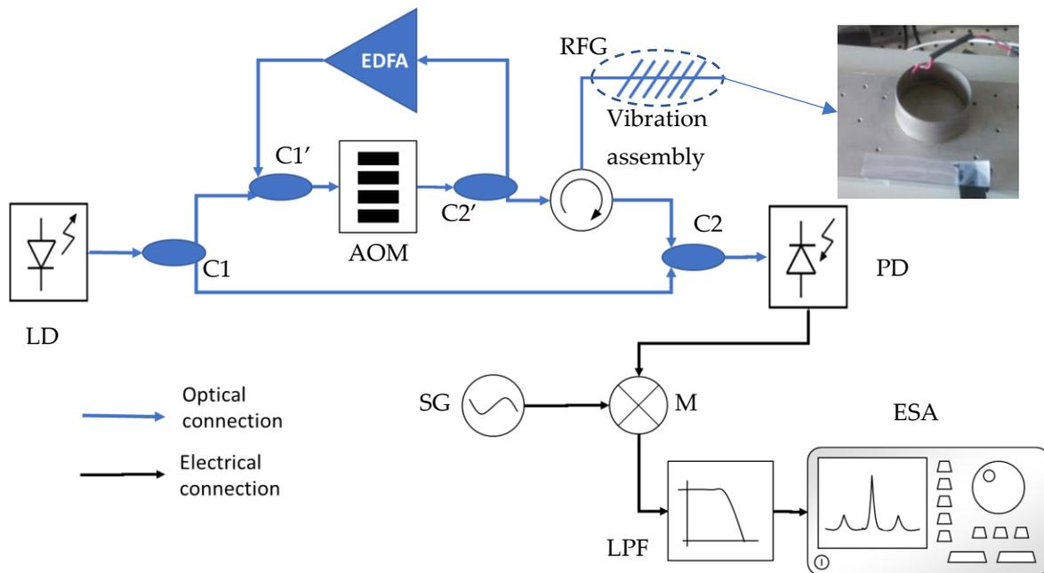
**Figure 2.** Self-heterodyne comb readout system together with the vibration assembly view. C1, C1', C2, C2': All couplers are 50:50 couplers. EDFA: erbium-doped fiber amplifier, AOM: acousto-optic modulator driven with a sinusoidal 200 MHz signal, LD: laser diode PD: photo-detector, LPF: low pass filter, ESA: electrical spectrum analyzer, SG: signal generator, M: mixer, RFG: random fiber grating.
