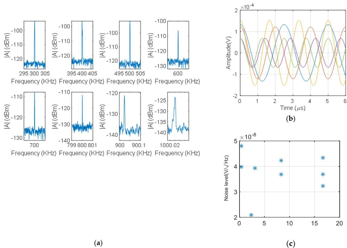
**Figure 6.** Measured output signals at different mechanical excitation frequencies over the random fiber grating: (a) the frequency domain of the signals, (b) time domain of the surface acoustic waves, (c) noise floor level for different bandwidth resolutions.
