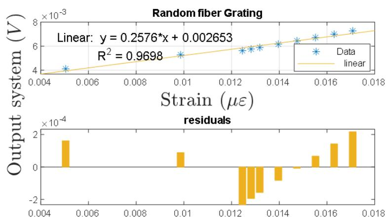
Figure 8. Response of the calibrating system to PZT strain excitation with output voltage.
