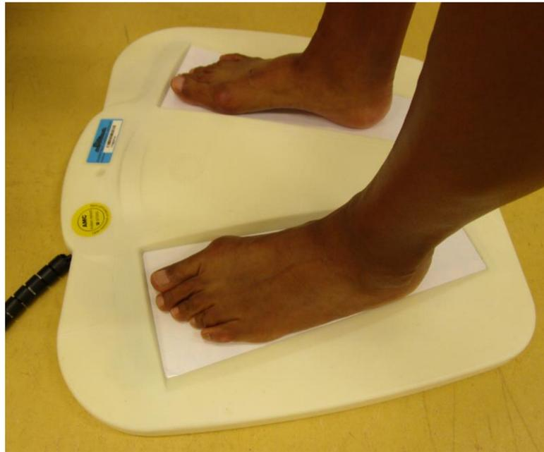
**Figure 1.** The foot temperature measurement platform system, showing the placement of the feet on the platform.
