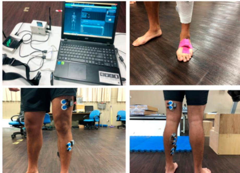
**Figure 1.** Full set-up position of IMU and EMG sensors.
