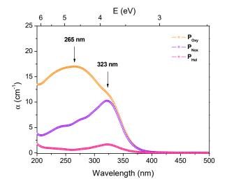
Figure 2. Ce-doped preforms optical absorption spectra.
