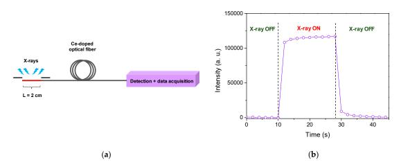
**Figure 7.** (a) Basic representation of the experimental setup used to evaluate the RL response of the Ce-doped optical fiber partially exposed to X-ray beam. (b) RL signal evolution versus time under 19.6 Gy(SiO<sub>2</sub>)/s dose rate.
