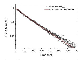
**Figure 4.** PL decay curve recorded on  $P_{Nox}$  at 450 nm wavelength, under excitation at 320 nm and its corresponding curve fitting analysis using Equation (1).
