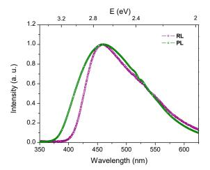
**Figure 9.** Ce-doped optical fiber responses: normalized typical RL spectrum and the PL one obtained under 320 nm excitation.
