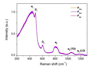
**Figure 1.** Raman spectra of the three Ce-doped preforms showing the band attribution according to ref. [30].
