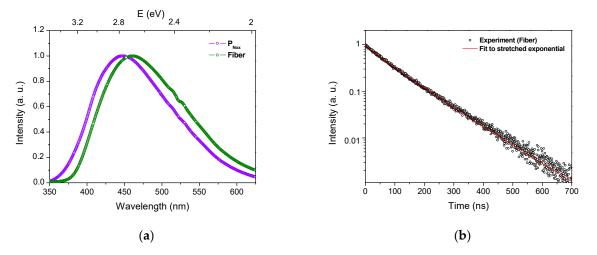
**Figure 6.** (a) Normalized PL spectra of Ce-doped optical fiber and its corresponding P<sub>Nox</sub> preform under 320 nm laser excitation. (b) PL decay curve at 450 nm, after probe excitation at 320 nm and a fit using Equation (1).
