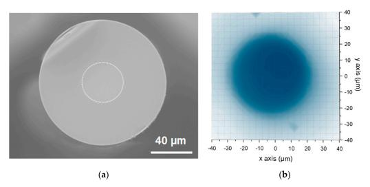
**Figure 5.** (a) SEM image of cross-section of the drawn fiber (the Ce-doped zone has been indicated by a white dashed circle), (b) Experimental mapping response of the Ce luminescence distribution along the fiber transverse cross-section: a laser excitation at 325 nm and a spatial step of 2.5 μm.
