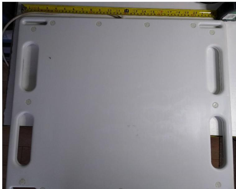
**Figure 12.** The assembled aluminum coil array in its Ertalyte enclosure.
