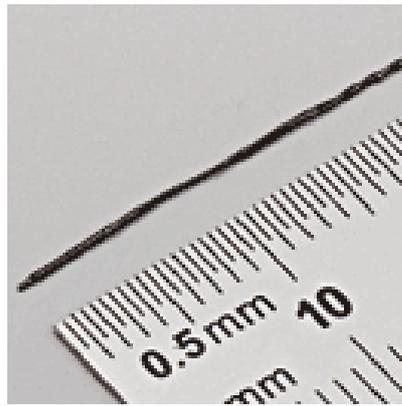
**Figure 9.** An example of the sensors used in this experiment, an Aurora 5-DOF sensor by NDI.
