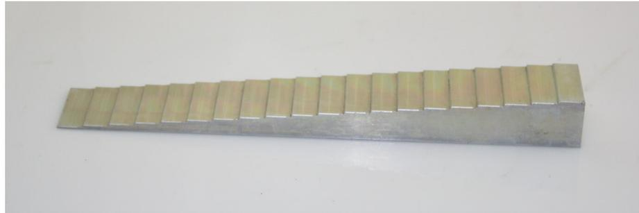
**Figure 14.** A pure aluminum step wedge was used as an X-ray absorption reference. This is a staircase profile aluminum block that increments in steps of 1 mm from 1–20 mm and is frequently used in the calibration and testing of X-ray systems.
