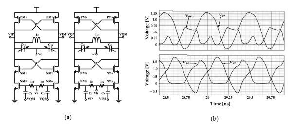
**Figure 7.** CMOS QVCO with split current sources: (a) schematic of the QVCO; (b) simulated waveforms at the drain–source and gate-source voltages of NM5 (top) and NM1 (bottom) (reproduced with permission from the author, Low phase noise self-switched biasing CMOS LC Quadrature VCO; published by IEEE, 2009) [52].
