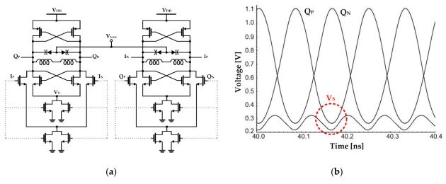
**Figure 5.** CMOS quadrature-VCO (QVCO) with separate current sources based on the switched-biasing technique: (a) schematic of the QVCO; (b) simulation waveforms at the outputs of the quadrature channel and the common node (reproduced with permission from the author, Low-phase-noise CMOS quadrature VCO; published by IEEE, 2006) [57].
