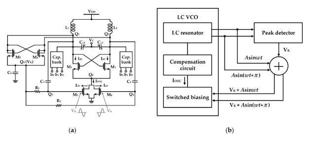
**Figure 13.** VCO using self-biasing with the adaptive DC voltage: (a) schematic; (b) operation of the self-biasing with the adaptive DC voltage from peak tracking at the oscillator outputs (reproduced with permission from the author, Low voltage CMOS LC VCO with switched self-biasing; published by Wiley, 2009) [63].
