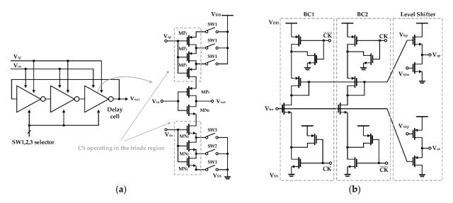
**Figure 4.** Ring VCO based on a switched-bias circuit (SBC): (a) block diagram of the ring VCO and schematic of the delay cell in the VCO; (b) schematic of SBC for current source modulation (reproduced with permission from the author, Low-voltage, low-phase-noise ring voltage-controlled oscillator using 1/f-noise reduction techniques; published by The Japan Society of Applied Physics, 2007) [50].
