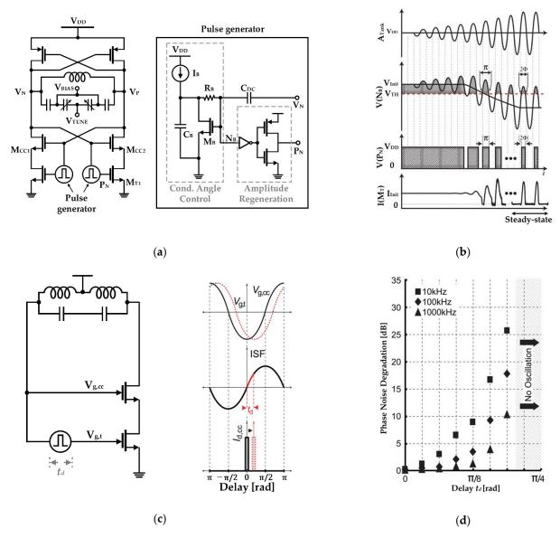
**Figure 14.** VCO employing the pulse generator that supplies pulse waveforms and the adaptive DC bias voltage: (a) schematic; (b) conceptual diagram of the VCO including the pulse generator operation; (c) intrinsic delay of the pulse generator; (d) simulated phase noise degradation with increasing the delay of the pulse generator (reproduced with permission from the author, A pulse-tail-feedback LC-VCO with 700 Hz flicker noise corner and −195dBc FoM; published by IEICE, 2019) [64].
