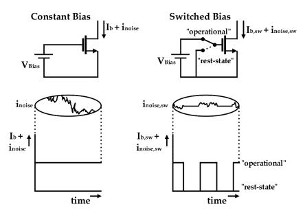
**Figure 1.** Conceptual diagram of switched-biasing technique (reproduced with permission from the author, reducing MOSFET 1/f noise and power consumption by switched biasing; published by IEEE, 2000) [33].
