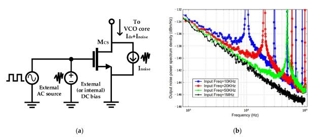
**Figure 15.** Characteristic of external-biasing topology: (a) conceptual schematic of external biasing (also available in PMOS configuration); (b) large noise peaks appearing as harmonics of the modulation frequency correlated with the external signal (reproduced with permission from the author, Experimental study on MOSFET's flicker noise under switching conditions and modelling in RF applications; published by IEEE, 2001) [56].
