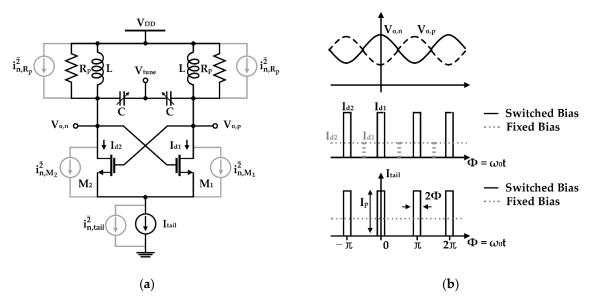
**Figure 3.** Analysis of VCO characteristics depending on the pulse modulation of the current source using the impulse sensitivity function theory: (a) schematic of the differential LC-VCO; (b) conceptual waveforms of the output voltages and drain currents of the VCO and the bias current by the pulse-modulated current source (reproduced with permission from the author, Tail current-shaping to improve phase noise in LC voltage-controlled oscillators; published by IEEE, 2006) [47].
