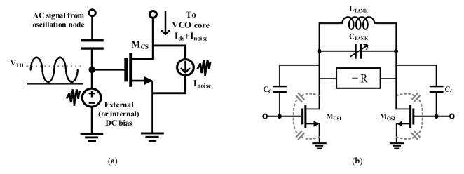
**Figure 16.** Characteristics of the self-biasing topology: (a) description of the self-biasing; (b) tuning range limit by the effect of the parasitic capacitances present at the current sources.
