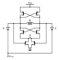
**Figure 2.** Schematic of a CMOS LC-VCO with the switched-biasing technique to the current source (reproduced with permission from the author, RF CMOS low-phase-noise LC oscillator through memory reduction tail transistor; published by IEEE, 2004) [34].
