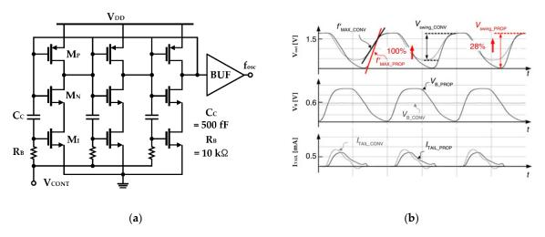
Figure 12. Ring VCO using the switched-biasing technique: (a) schematic; (b) simulated waveforms of the VCO output (top), bias voltage of the current source (middle), and tail current of the inverter cell (bottom) (reproduced with permission from the author, Low phase noise ring VCO employing input-coupled dynamic current source; published by IET, 2020) [61].
