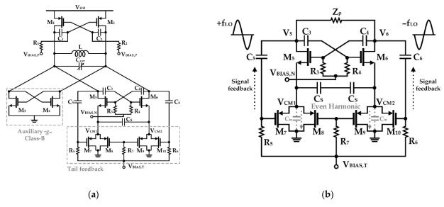
**Figure 11.** Class-C CMOS VCO using the switched-biasing technique: (a) schematic of the VCO; (b) bias conduction at the sub-threshold operation of the split current sources implemented by PMOS transistors (reproduced with permission from the author, A 2.2 to 2.9 GHz complementary class-C VCO with PMOS tail-current-source feedback achieving—120 dBc/Hz phase noise at 1 MHz offset; published by IEEE, 2019) [54].
