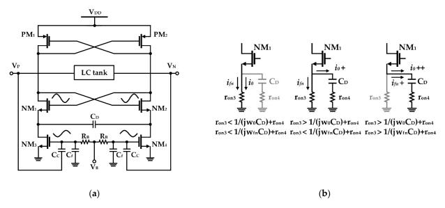
**Figure 8.** CMOS VCO including degeneration and filter capacitors: (a) schematic of the VCO; (b) current flows depending on the capacitance of CD—the usage of the optimal capacitance can divide the current into two paths, as shown in the middle case (reproduced with permission from the author, Reduction of  $1/f^3$  phase noise in LC oscillator with improved self-switched biasing; published by Springer, 2015) [58].
