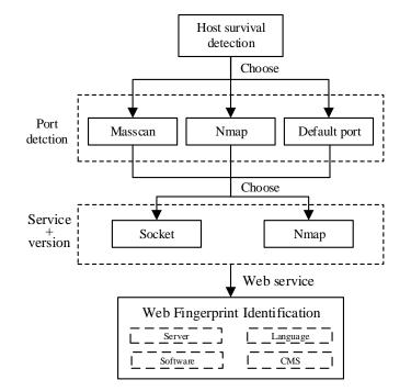
Figure 4. Network asset identification diagram.
