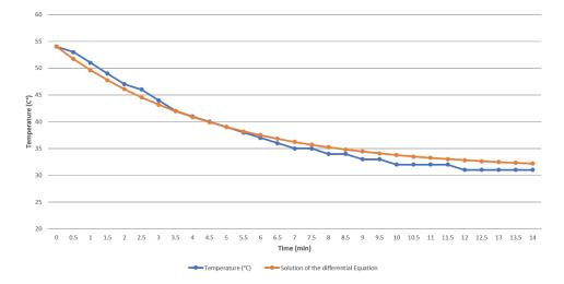
Figure 12. Measured temperature and temperature obtained with the solution of the differential equation.
