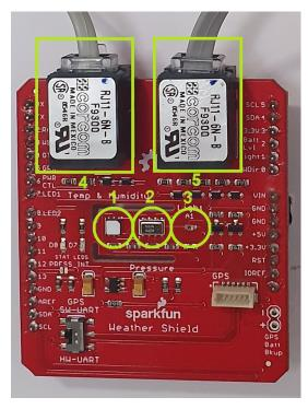
Figure 5. MEIoT Weather Station sensors.
