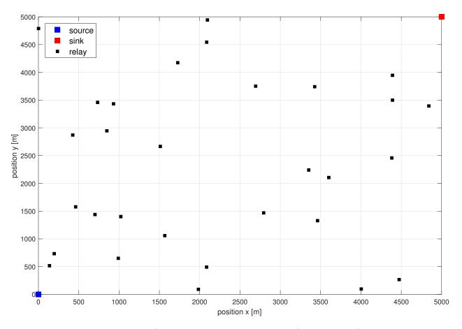
Figure 2. Example of the network topology with 30 relays, for area width of 5 km.
