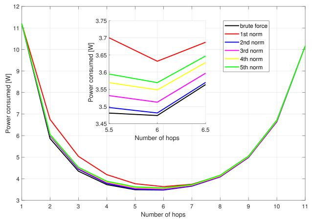
Figure 3. Power consumption of the network with 10 relays for area width of 5 km.
