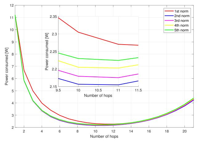
Figure 5. Power consumption of the network with 30 relays for area width of 5 km.
