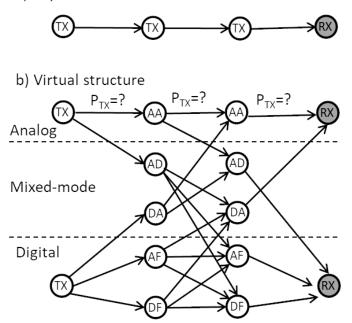
**Figure 1.** Diagram of the physical and virtual structure of the optimized subnetwork. AA: analog relay, AD: analog-digital relay, DA: digital-analog relay, AF: amplify and forward digital relay, DF: decode and forward digital relay.
