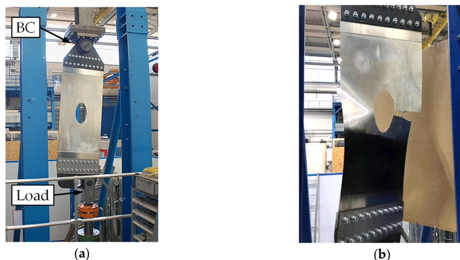
Figure 9. (a) test setup for demonstrator; (b) failed structure.
