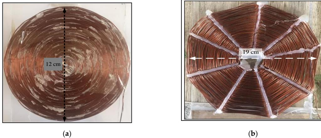
**Figure 3.** Types of coils (a) spiral coil and (b) spider coils.
