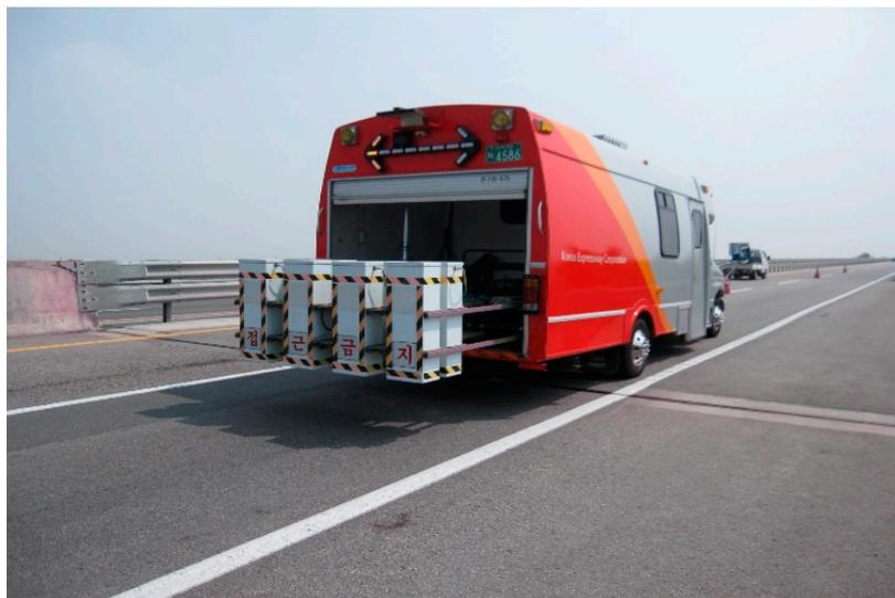
**Figure 2.** Photo of a GPR survey vehicle using 4-channel 1 GHz air-coupled antennas.
