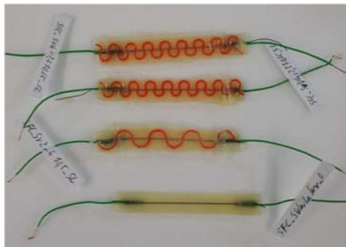
**Figure 1.** Different embedded sensor systems with (top) and without (bottom) the embedded support spring structure.
