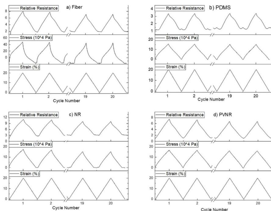
**Figure 3.** First and last two cycles of 20 cyclic stretches from 0% to 20% for (a) the single fiber and the sensor fiber embedded in (b) PDMS, (c) natural rubber (NR) and (d) pre-vulcanized natural rubber (PVNR).
