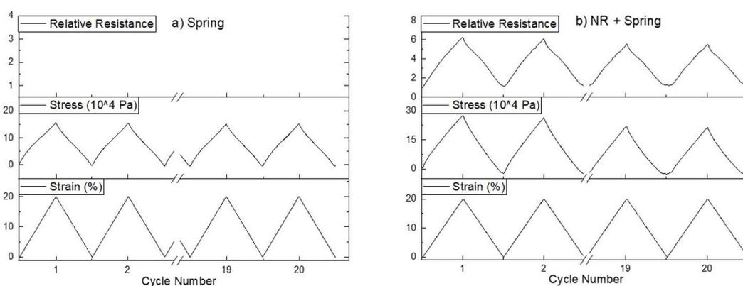
**Figure 4.** Twenty cyclic stretches from 0% to 20% for (a) the 3D printed spring structure and (b) the piezoresistive composite with natural rubber as casting material and the 3D printed spring of which the first and last two cycles are shown.
