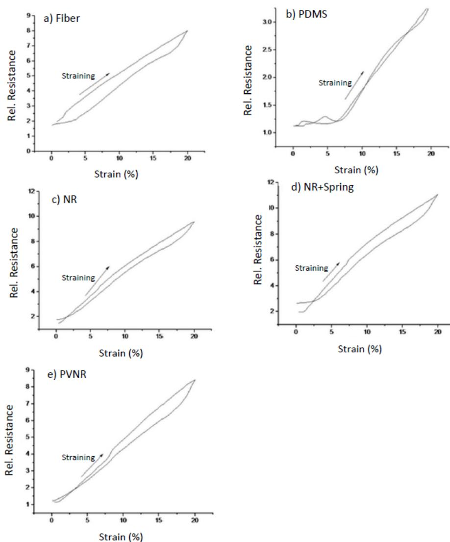
**Figure 6.** The relative resistance as a function of the strain during the first cycle of the dynamic testing for (a) the single fiber and the fiber embedded in (b) PDMS, (c) natural rubber (d), natural rubber with the spring structure and (e) pre-vulcanized natural rubber.
