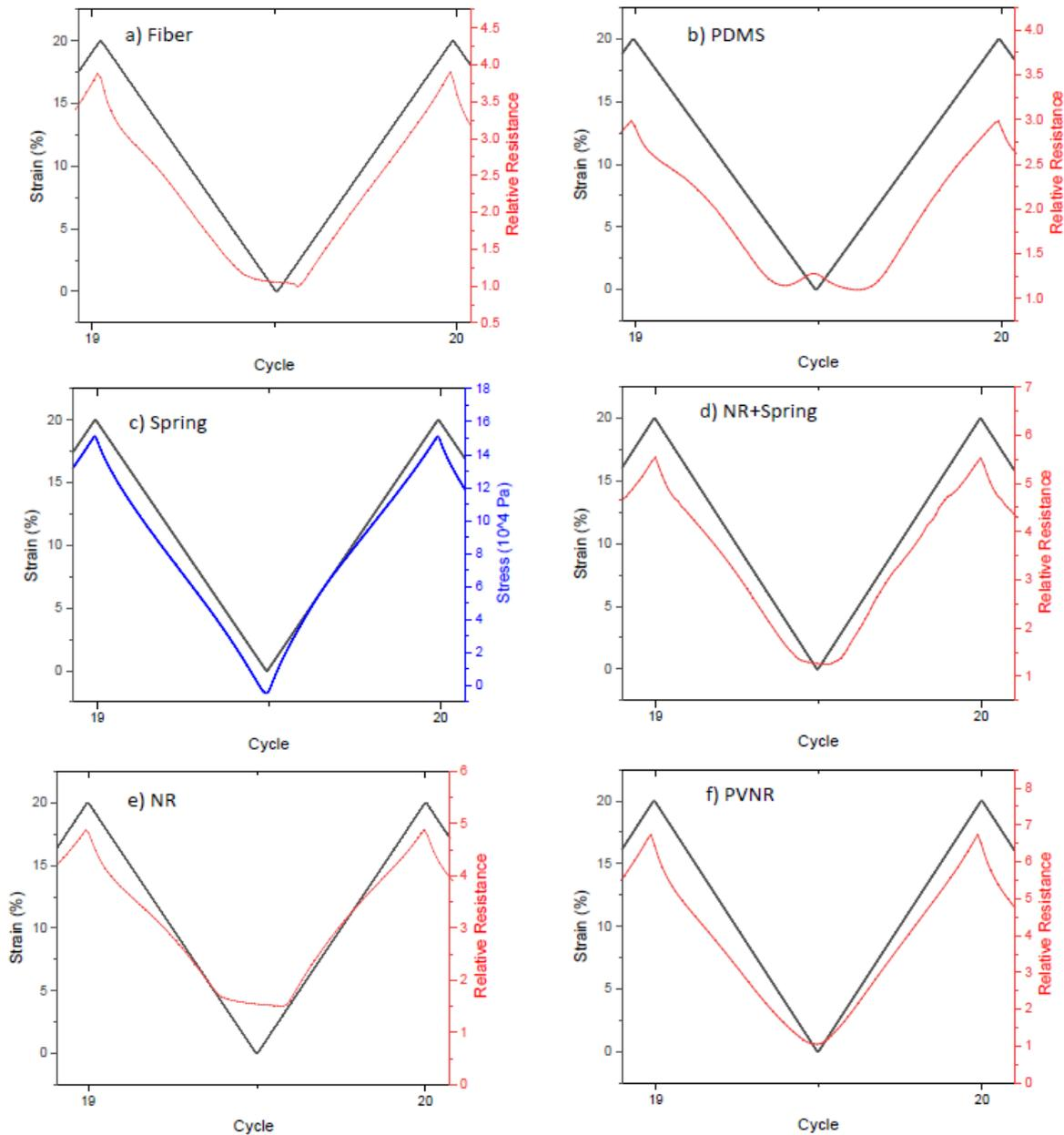
**Figure 5.** Overview of the electrical resistance (a,b,d,e,f) for the fiber sensor composites and the mechanical response of the 3D printed spring structure (c) between the 19th and 20th cycle of the cyclic tensile test.
