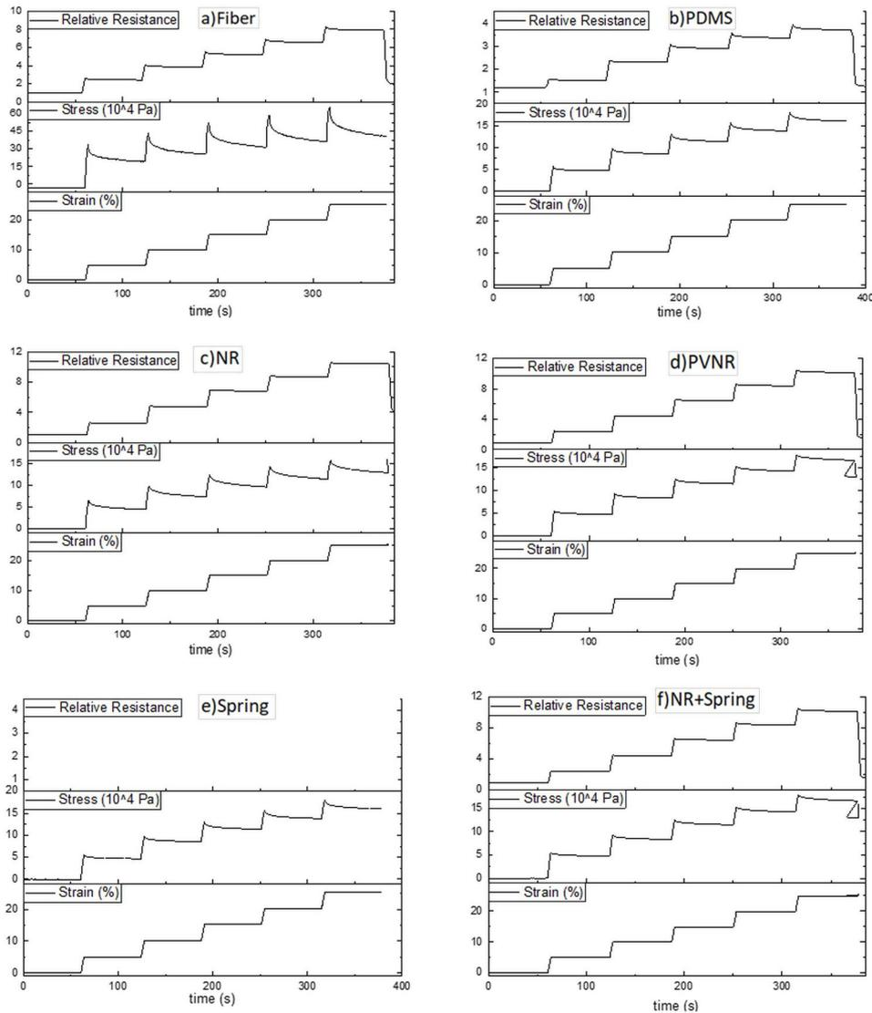
**Figure 8.** Quasi-static stepwise tensile test for (a) the single fiber, the fiber embedded in the elastomer (b) PDMS, (c) natural rubber, (d) pre-vulcanized natural rubber, (e) the spring structure and (f) the fiber embedded in natural rubber with the spring structure.
