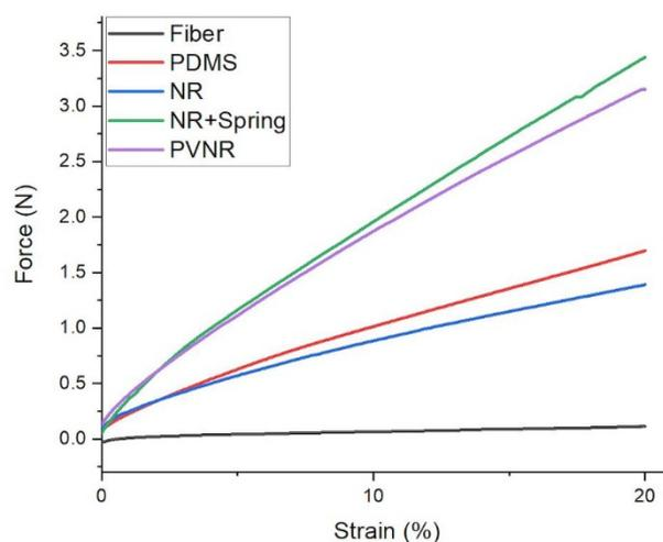
**Figure 9.** Tensile force vs. strain behavior of single piezoresistive (grey solid line) fiber and different fiber embedded sensor materials between 0 % and 20 % during the first cycle of the cyclic tensile test.
