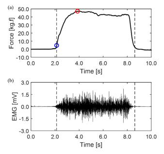
**Figure 4.** Example signal of muscle fatigue measurement. (**a**) load cell force data, red circle: 100% peak force, blue circle: 10% peak force. (**b**) biceps electromyogram (EMG) data.
