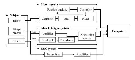
Figure 2. The continuous passive motion mirror therapy (CPM-MT) system overview.
