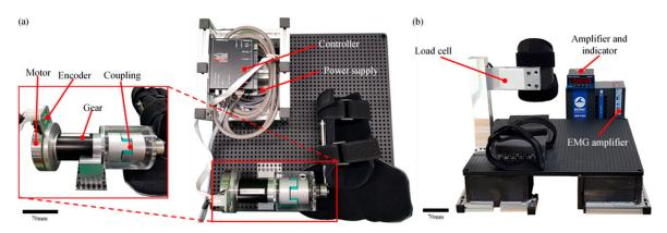
**Figure 1.** (a) The continuous passive motion mirror therapy (CPM–MT) system comprises coupling, gear, motor, encoder, controller, and power supply. (b) The muscle fatigue measurement system comprises load cell, load cell amplifier, indicator, and electromyogram (EMG) amplifier.
