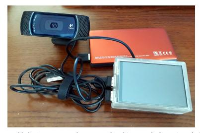
**Figure 4.** The assembled microcomputer that was used in this research. It consists of a Raspberry Pi 3 model B+ in a semi-transparent case with a 3.5" LCD touchscreen, a Logitech Webcam C920 HD Pro, and a powerbank (5 V, 3 A).
