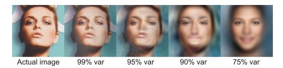
**Figure 3.** Actual (input) image and its reconstruction using various numbers of eigenfaces, which describe 99%, 95%, 90%, and 75% of variance, respectively.
