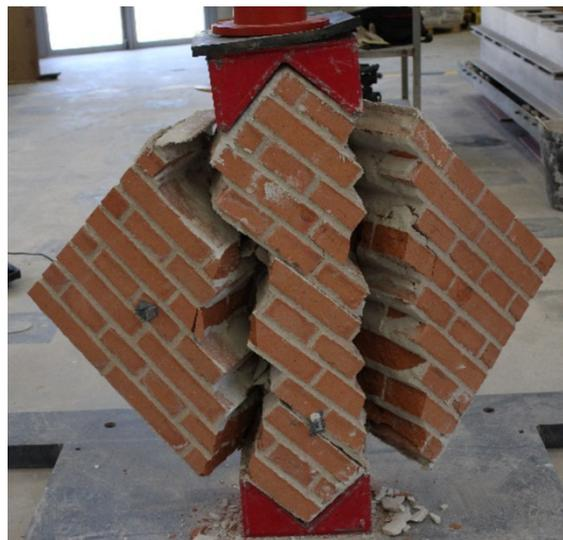
**Figure 13.** Tilting towards the reinforced in single-reinforced (2) specimen.
