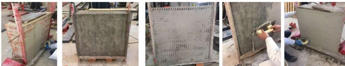
**Figure 4.** Illustration of the retrofitting of masonry specimens with textile-reinforced mortar (TRM) in the laboratory.
