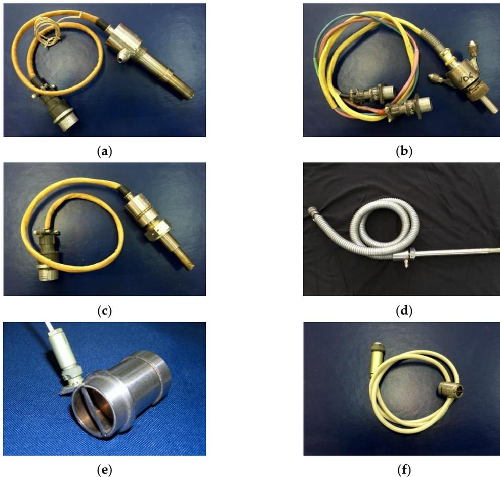
**Figure 3.** Examples of SCECS for RC measuring in a GTE turbine with forced air (a) and liquid (b) cooling; in a GTE compressor (c); in shaft seals (d); in a ducted propfan (e) and in GTE support bearings (f).
