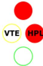
Figure 14. Alarm of GNSS fault—position or *HPL* not available, conceptual presentation in ECDIS.
