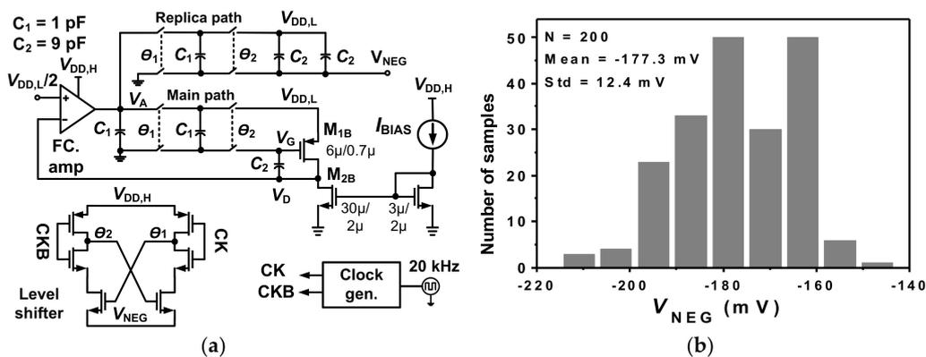
Figure 4. (a) Schematic of the negative voltage generator, (b) statistical distribution of  $V_{NEG}$ .
