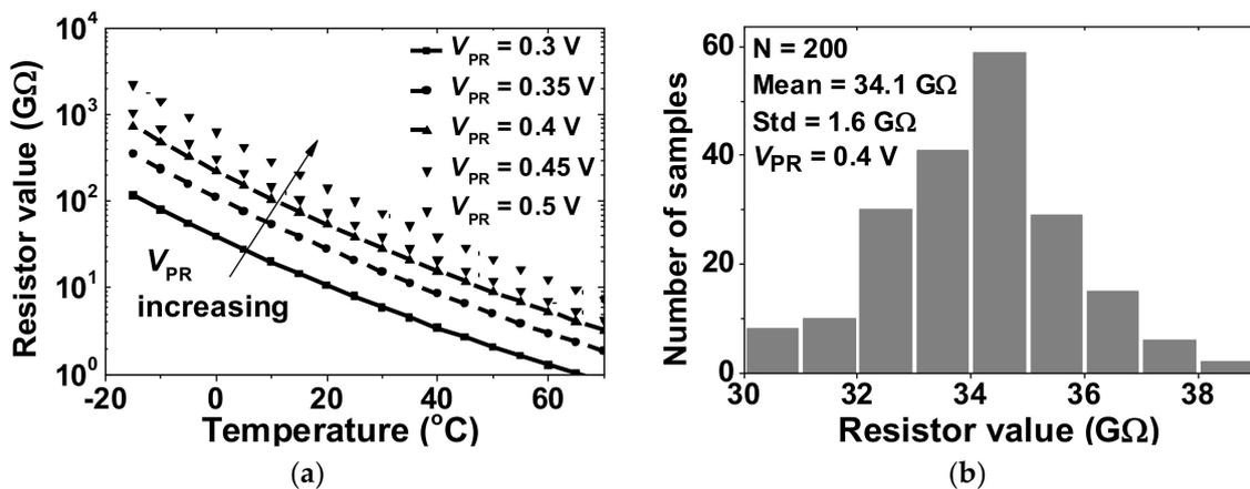
Figure 8. (a) simulated value of the pseudo-resistor as a function of temperature for various  $V_{PR}$  and (b) Monte Carlo simulation result of the pseudo resistor value at  $V_{PR} = 0.4$  V.
