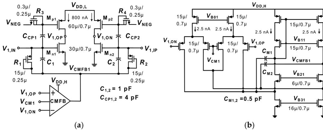
Figure 3. (a) Schematic of the squeezed-inverter stage using the shared common-mode feedback (CMFB).  $V_{CM1} = 0.1$  V,  $V_{NEG} = -0.18$  V, and  $V_{CMFB1} = 0.098$  V (nominal value). (b) Schematic of the proposed CMFB circuit.  $V_{B01} = 0.57$  V,  $V_{B11} = 0.28$  V,  $V_{B21} = 0.49$  V, and  $V_{B31} = 0.23$  V.
