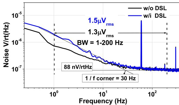
Figure 15. Measured input-referred noise voltage spectral density.
