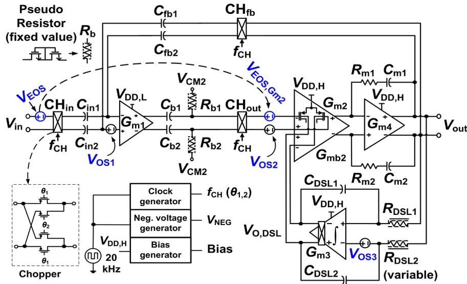
**Figure 1.** Schematic of the proposed capacitively-coupled chopper instrumentation amplifier (CCIA) using body-controlled DC servo loop (DSL).  $C_{in1,2} = 4$  pF,  $C_{fb1,2} = 40$  fF,  $C_{b1,2} = 3$  pF,  $C_{m1,2} = 4$  pF,  $R_{m1,2} = 4$  M $\Omega$ , and  $C_{DSL1,2} = 5$  pF.
