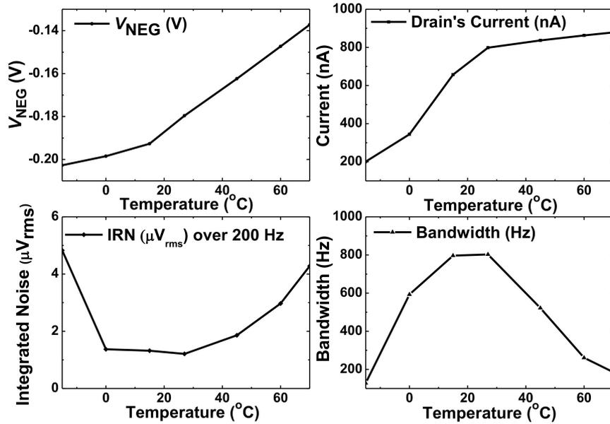
**Figure 11.** Simulated bias current, noise, and bandwidth depending on temperature.
