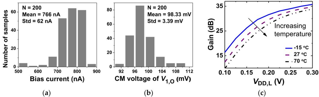
**Figure 5.** Monte Carlo simulation results for the (a) bias current, (b) output common-mode (CM) voltage of the squeezed-inverter (SQI) stage. (c) simulated gain of the SQI stage depending on  $V_{DD,L}$  and temperature.
