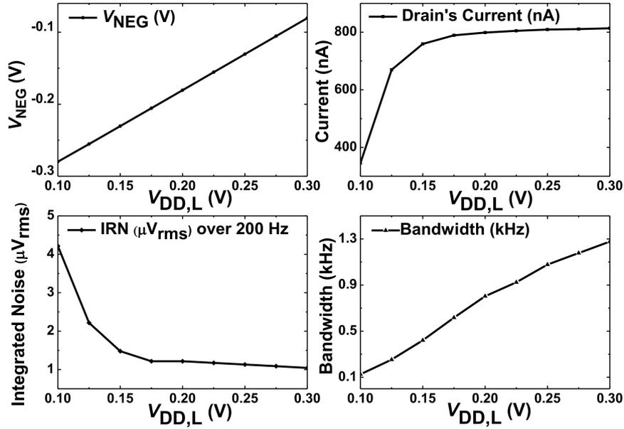
**Figure 10.** Simulated results showing the effect of  $V_{\text{DD,L}}$  on the noise and bandwidth of the proposed CCIA.
