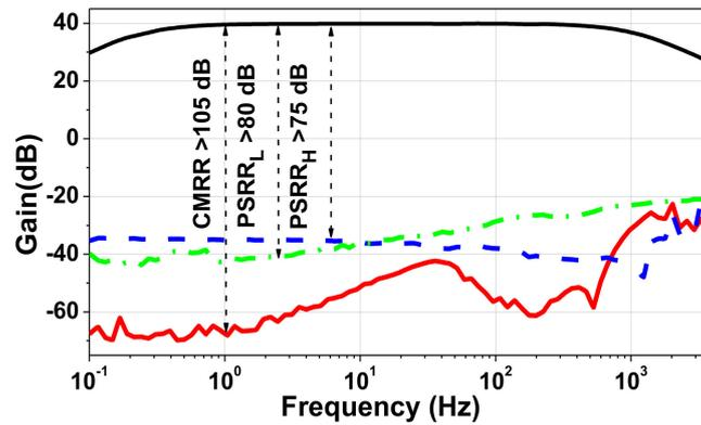
Figure 14. Measured CMRR and power supply rejection ratio (PSRR) as a function of frequency.
