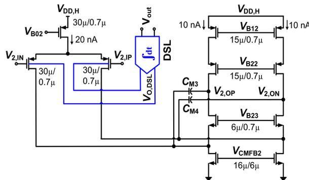
**Figure 6.** Schematic of transconductor  $G_{m2}$  with body-controlled DSL.  $C_{M3,4} = 0.5$  pF.  $V_{B02} = V_{B12} = 0.52$  V,  $V_{B22} = 0.18$  V,  $V_{B23} = 0.6$  V, and  $V_{CMFB2} = 0.28$  V (nominal value).
