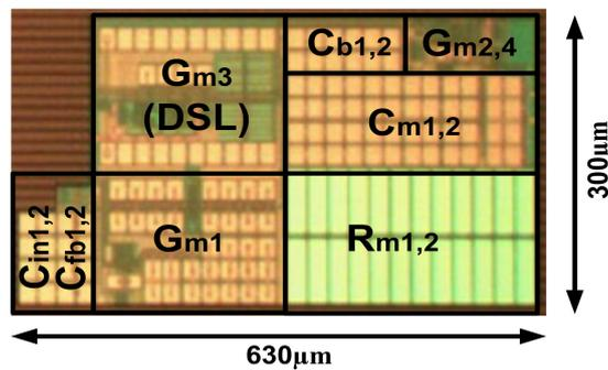
Figure 12. Chip microphotograph of the proposed CCIA.
