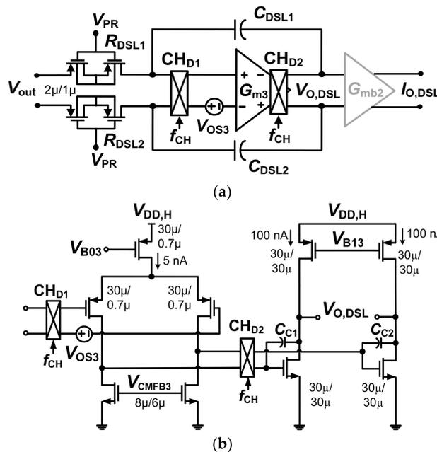
**Figure 7.** (a) schematic of the DSL and (b) schematic of the two-stage opamp  $G_{m3}$ .  $C_{DSL1,2} = 5$  pF,  $C_{C1,2} = 0.5$  pF.  $V_{B03} = 0.57$  V,  $V_{B13} = 0.34$  V, and  $V_{CMFB3} = 0.29$  V (nominal value).
