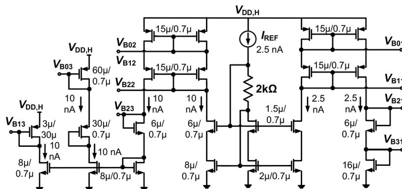
Figure 9. Schematic of the bias generator.
