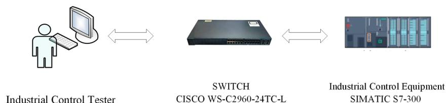
**Figure 8.** Experimental environment for vulnerability mining of Modbus TCP.
