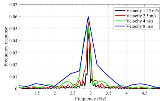
**Figure 13.** The frequency response of the middle of bridge under moving load with different velocities.
