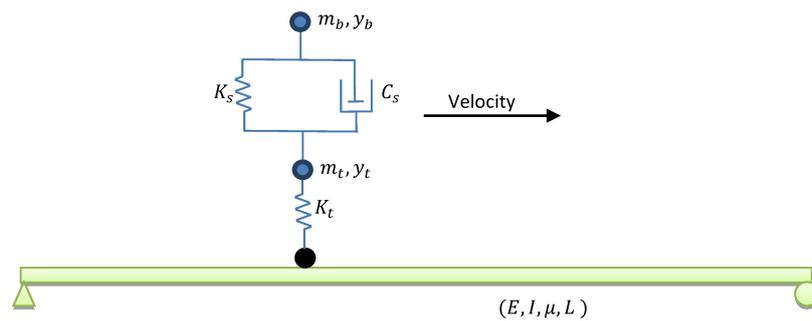
Figure 2. Schematic view of the simply supported beam under moving sprung mass.
