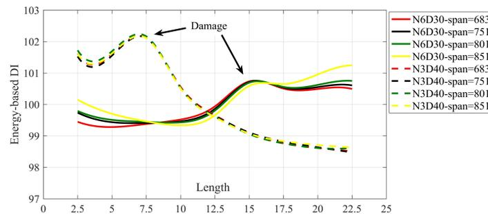
**Figure 11.** The spline of DIs for different application of SGF with unique span. All the results are for velocity = 1.25 m/s.
