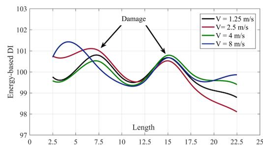
**Figure 7.** The spline of DIs along the bridge for the case of multi-damage, N3N6D40, with different velocities.
