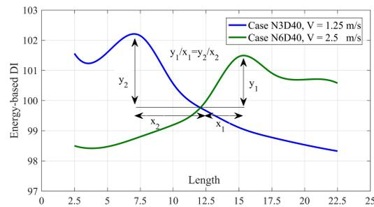
Figure 8. The schematic view of relative slope between the max of spline and the intersection point.
