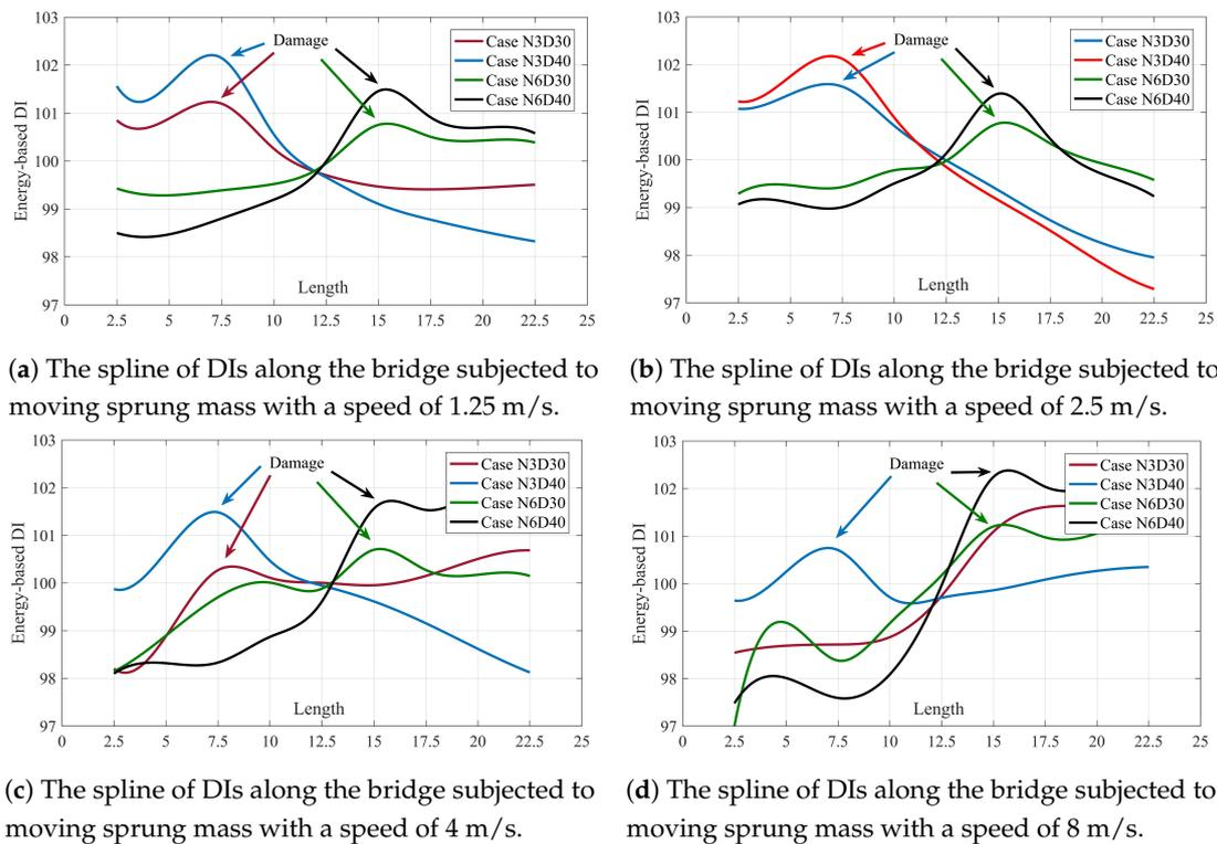
**Figure 6.** The spline of DIs along the bridge of different scenarios and different velocities. (a) velocity = 1.25 m/s, (b) velocity = 2.5 m/s, (c) velocity = 4 m/s, (d) velocity = 8 m/s.
