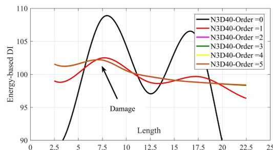
**Figure 12.** The spline of DIs for using SGF with different orders. All the results are for velocity = 1.25 m/s.
