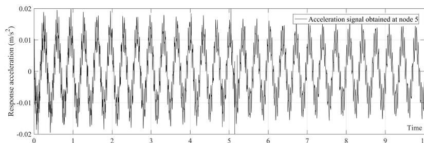
Figure 4. Acceleration response at the middle of the bridge under moving sprung mass with speed of 2.5 m/s.
