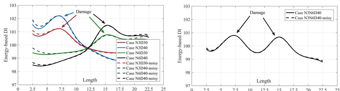
(a) The spline of noisy and noise-free DIs along the bridge subjected to moving sprung mass with a speed of 1.25 m/s for single-damage scenarios.
