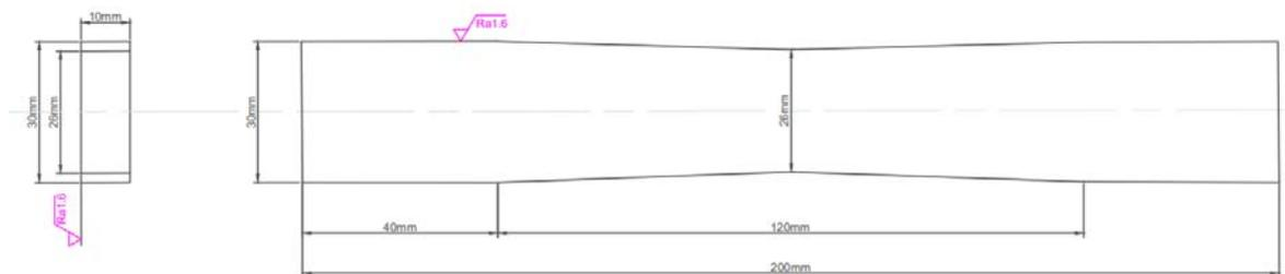
Figure 6. Dimensions of the test specimens.
