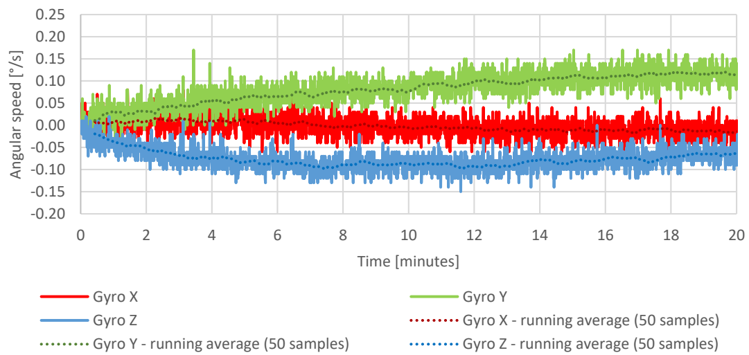
Figure 16. Stationary measurements of gyroscope drift.
