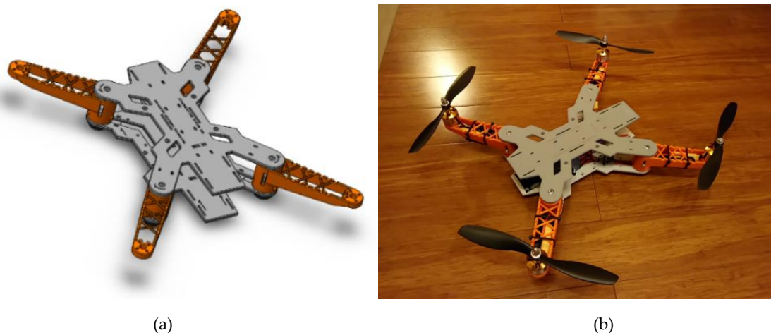
Figure 3. (a)—The 3D model of a quadcopter frame design [5], (b)—fully assembled quadcopter.
