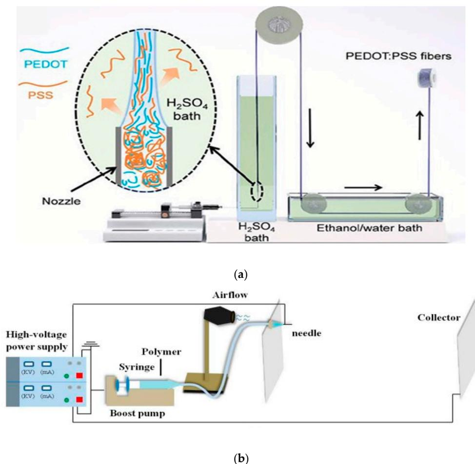
**Figure 3.** Fiber spinning process: (a) schematic illustration modified set-up used in wet-spinning PEDOT:PSS fibers. Inset shows the schematic illustration of the alignment of PEDOT:PSS chains during fiber formation and the outward diffusion of excess PSS to  $H_2SO_4$  coagulation bath. Adapted from [74]; (b) schematic diagram of electrospinning setup; the distance between the needle and collector was 120 cm. Adapted from [77].
