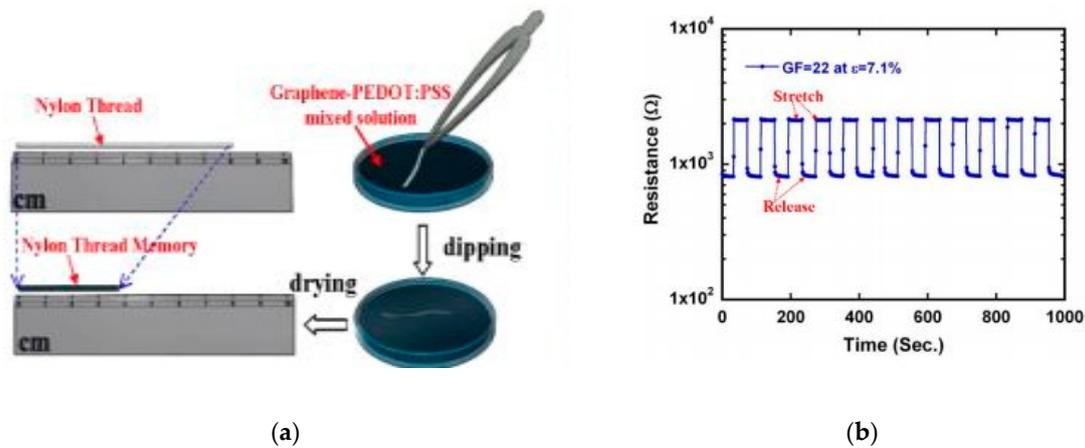
**Figure 7.** A graphene-PEDOT:PSS coated nylon thread: (a) schematic of the simple two-step dip-and-dry solution process for the fabrication (right) and the actual picture of the sample with the length reduction from 80 to 29.48 mm after dip-and-dry; (b) resistive memory strain sensor thread at many stretch and release cycle under applied a fixed  $\varepsilon = 7.1\%$ . Adopted from [92]
