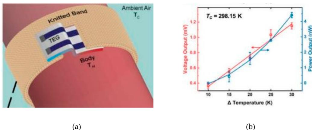
**Figure 8.** (a) Design schematic of a wearable thermoelectric generator; (b) thermoelectric power and voltage outputs for a tobacco cotton thermopile at  $25 \text{ }^\circ\text{C}$ . Adapted from [101].
