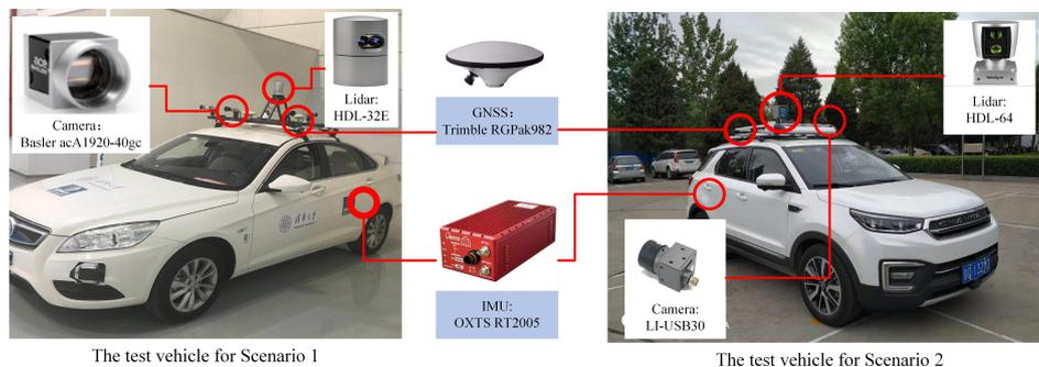
**Figure 13.** The experimental intelligent vehicles.
