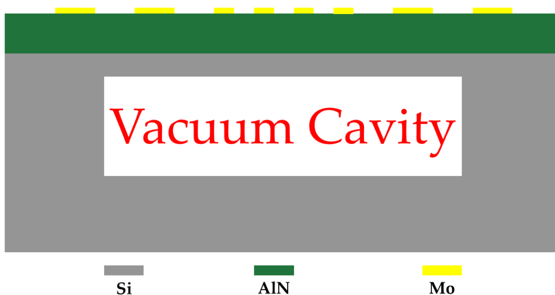
Figure 1. the cross-sectional view of a refreshed acoustic wave pressure sensor design with a deep vacuum cavity.
