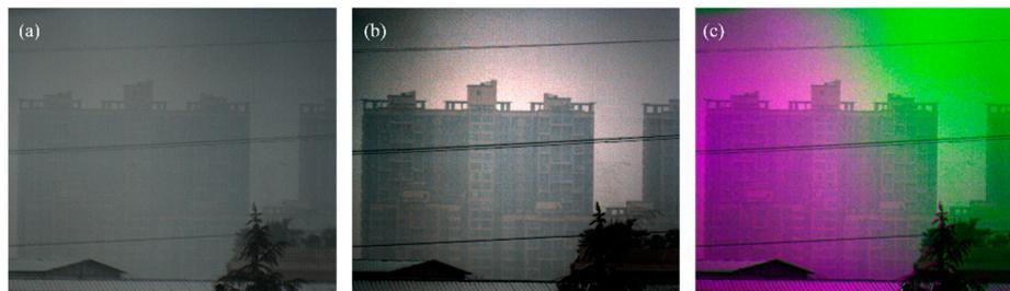
**Figure 7.** The dehazing experimental results. (a) Original intensity image; (b) dehazed image using the current proposed method; and (c) dehazed image using our previously proposed method with the fixed bias parameters.
