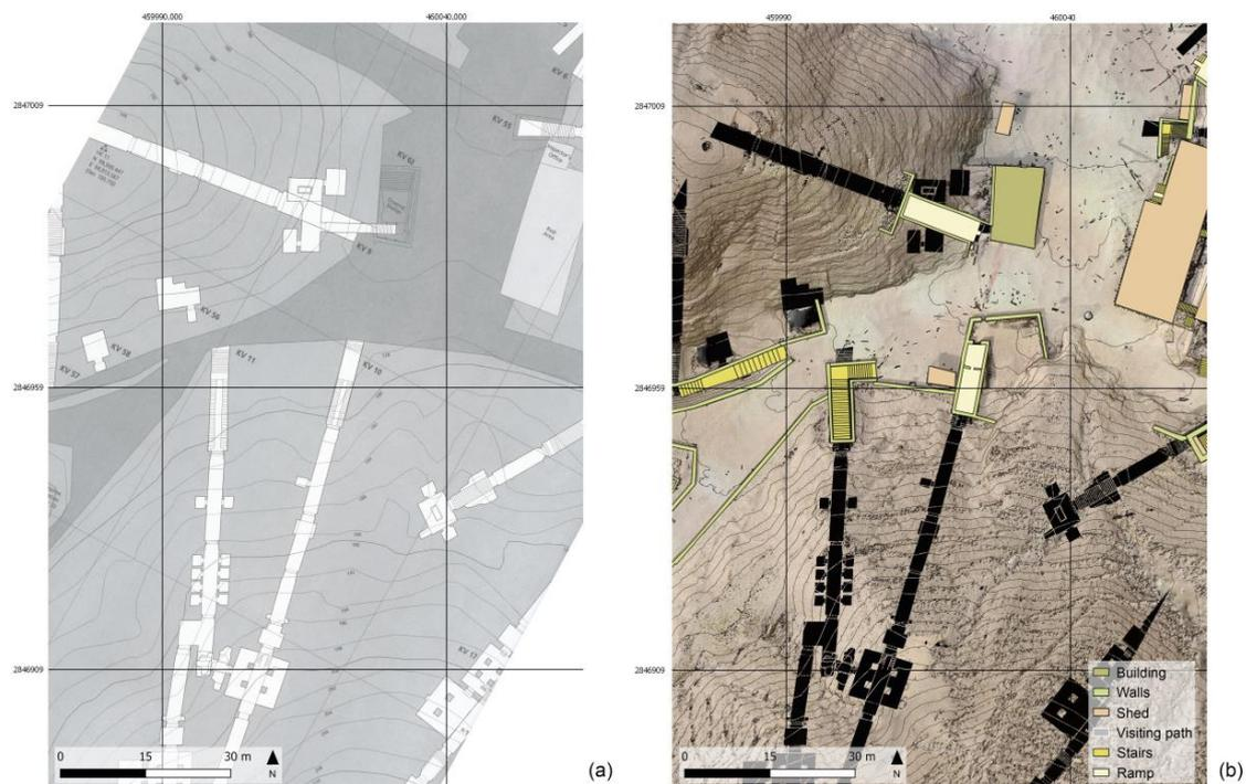
**Figure 11.** Different survey products and underground tombs derived from the Theban mapping project sheets integrated into the Geographic Information System (GIS) environment. (a) Sheet 5/70, KV (3/4) extracted from the Atlas of the TMP, page 21, with superimposed the new global grid (50 m interval), Plan 1:400, Contour interval 2 m; (b) the corresponding area with the up-to-date geoinformation in GIS environment, Plan 1:100, contour interval 1 m, same global grid as on the left.
