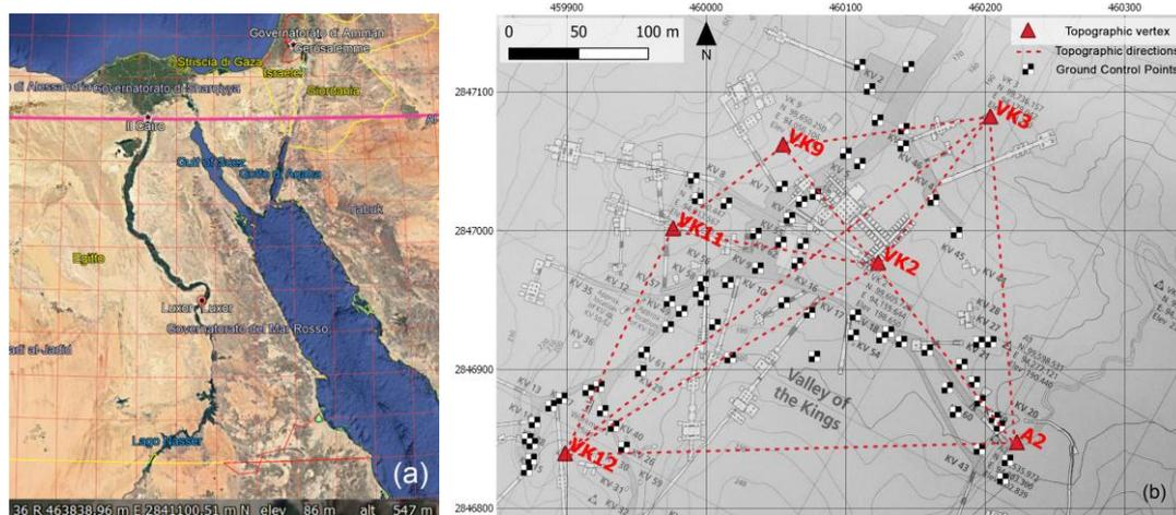
**Figure 1.** The Valley of Kings (VOK) in Luxor: (a) VOK location in UTM (source Google Earth). (b) The measured topographic network (red triangles) and the localization of Ground Control Points (black and white markers) derived from total station measurements, superimposed to the Sheet 1/70, KV and WV extracted from the Atlas of the Theban Mapping Project (TMP), page 13, Plan 1:2500, Contour interval 10 m.
