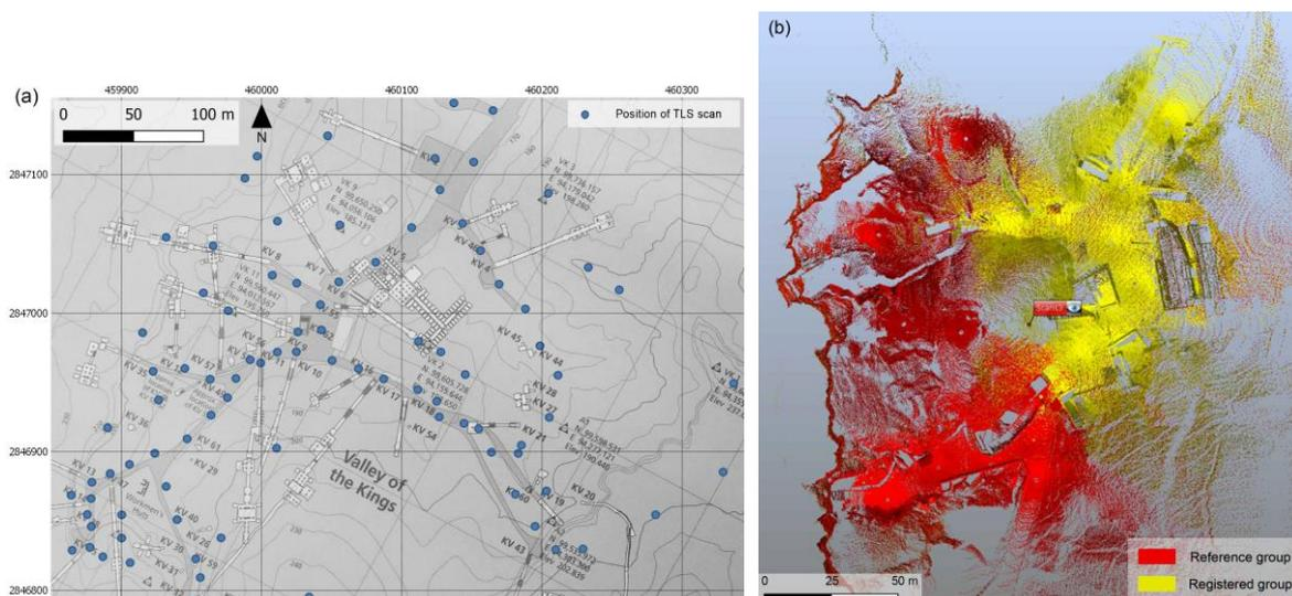
**Figure 2.** Laser scanning survey: (a) position of each of the acquired TLS scans (blue dots), superimposed to the Sheet 1/70, KV and WV extracted from the Atlas of the TMP, page 13, Plan 1:2500, Contour interval 10 m. (b) The registration process of the scans groups performed via the software Faro SCENE.
