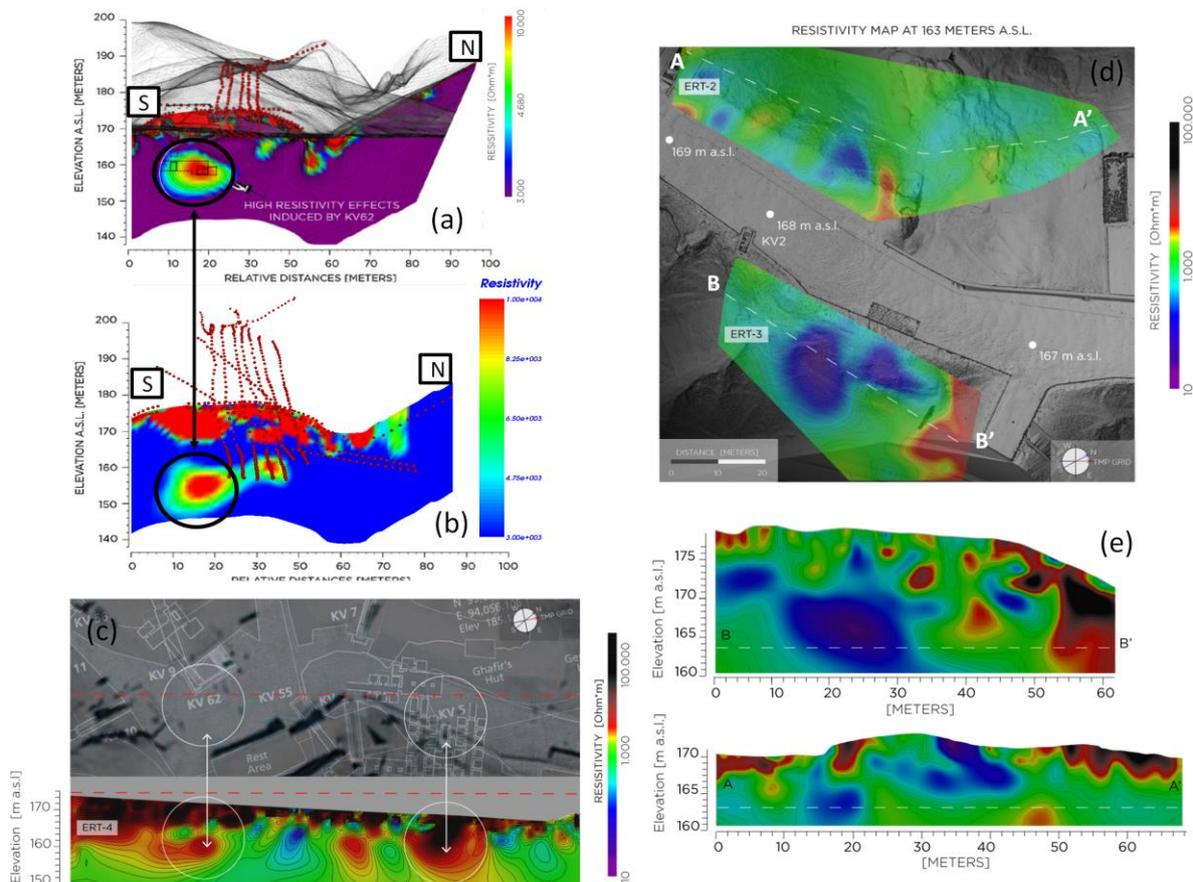
**Figure 14.** Results from ERT surveys: (a) and (b) representative cross-section of the 3D model over the KV62 tomb (a from 2017 surveys and b from 2018 surveys); (c) the electric resistivity variation reconstructed by ERT-4 and comparison with known voids. The electric resistivity variation reconstructed by ERT-2 and -3 shown by representative maps (d) and their associated cross-sections (e). Dashed white lines show where each map and its vertical section intersect.
