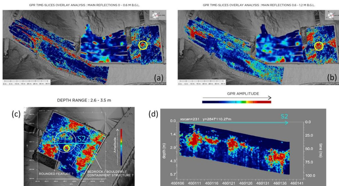
**Figure 15.** Results of GPR time slice overlay analysis over and around the KV2-A area. In (a) and (b) a sequence of time slices for two representative depth ranges is reported. In (c) and (d) a focus on the area in front of KV2 with: a time slice for a representative depth range (c) and the corresponding cross-section S2 (d) showing the distribution at depth of the main anomalies.
