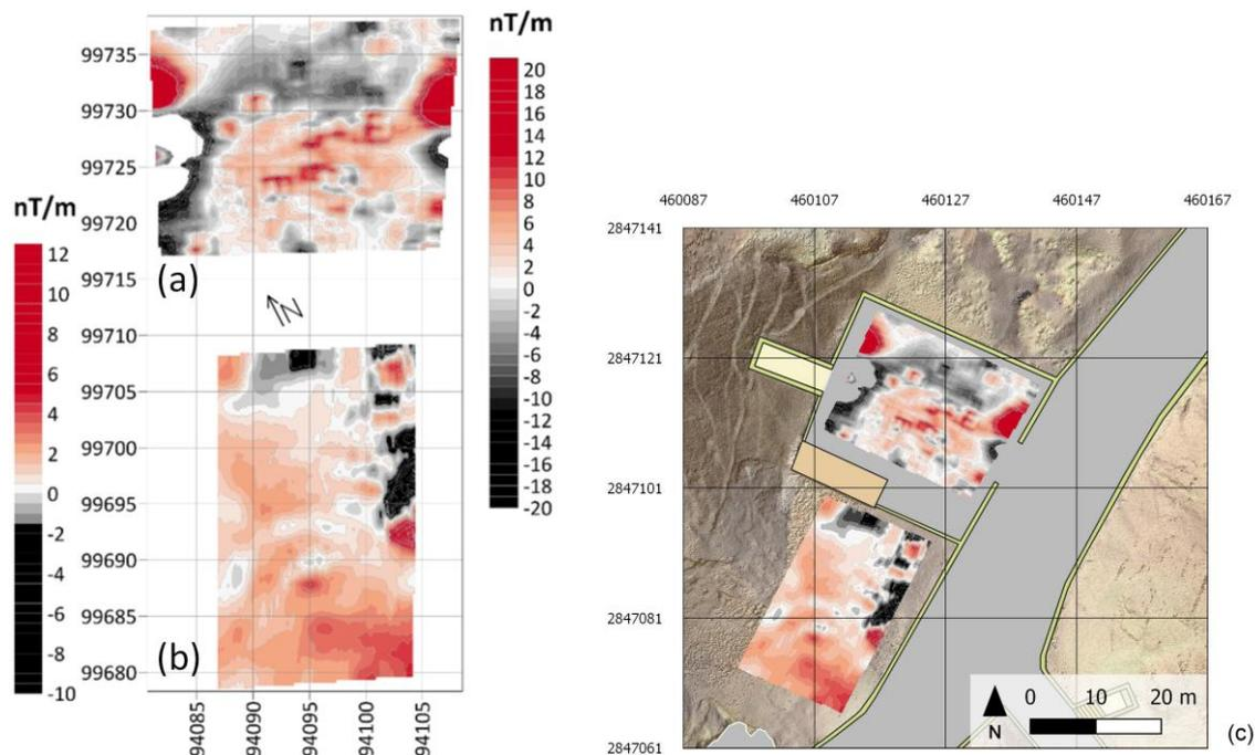
**Figure 16.** VGTMF map (local coordinates system) of (a) MAG-3 and (b) MAG-2 areas. The left color scale refers to MAG-2, the right color scale refers to MAG-3. The color scales have different ranges to enhance the peculiarity of the two areas. In (c) the same VGTMF maps are integrated in the geomatics GIS environment (georeferenced in the UTM WGS 84 system).
