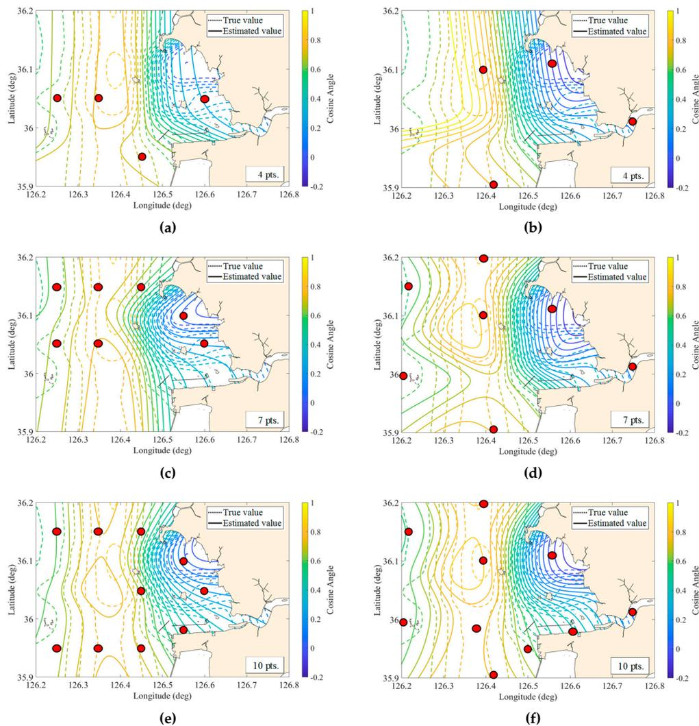
**Figure 5.** Comparison of the spatial distribution between true and estimated field reconstructed by using 4 (a,b), 7 (c,d), and 10 (e,f) points of the monitoring array, based on the quantitative optimization (left) and graphical optimization (right).
