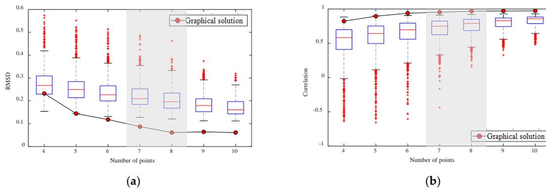
**Figure 7.** (a) Root mean square differences (RMSDs) and (b) correlation coefficient (CORs) of spatial distribution reconstructed by array of quantitative and graphical optimization.
