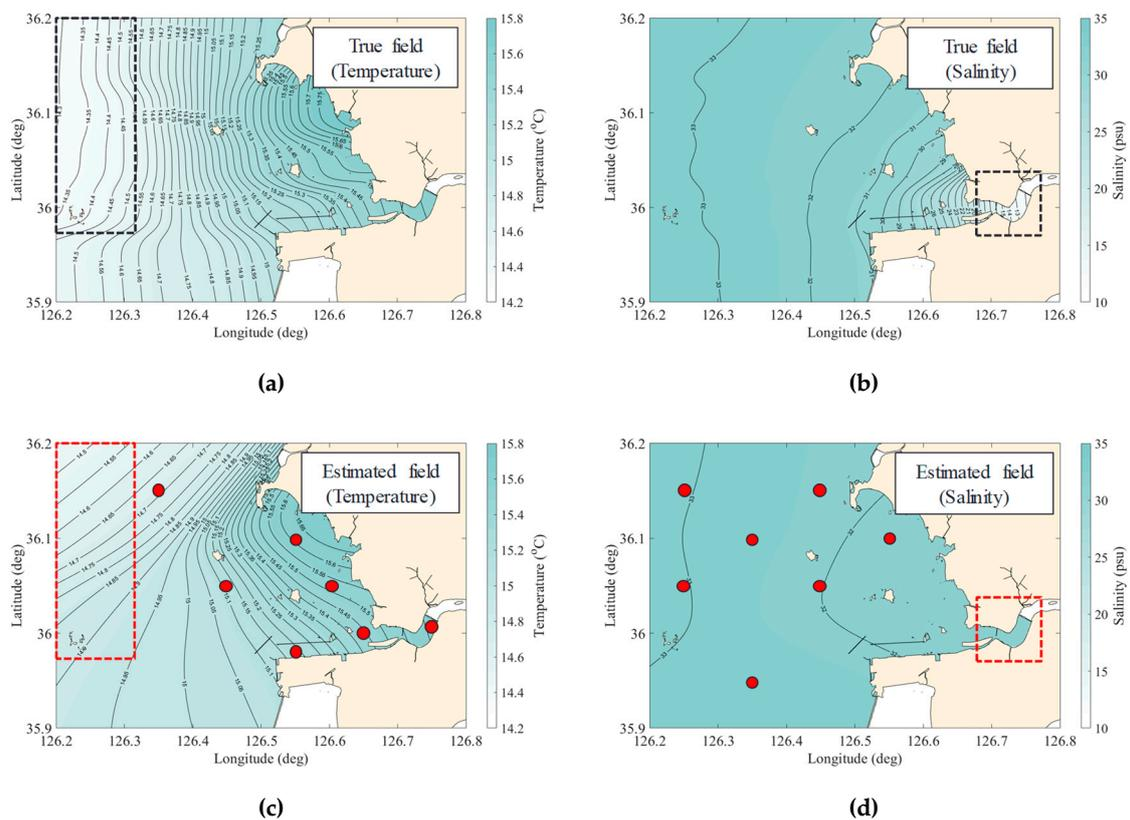
**Figure A1.** The true field of (a) water temperature and (b) salinity, and the example of the monitoring array (c) designed by considering only salinity and reconstructing the spatial distribution of the water temperature, and (d) designed by considering only water temperature and reconstructing the spatial distribution of the salinity.
