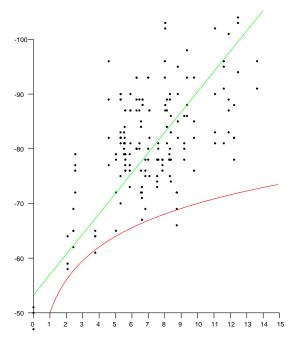
**Figure 1.** Scattergram of Signal Strength (RSS) versus distance in typical three-level wooden building. Horizontal axis: distance between smartphone and Wi-Fi access points (APs) (in meters). Vertical axis: Signal Strength (in dBm). Red curve: expected inverse square law dependence  $(-50 - 20 \log(R) \text{ dBm})$ . Green line: linear fit (-53 - 3.7 R dBm). Because of the large scatter, it should be clear that RSS is not very useful for estimating distance.
