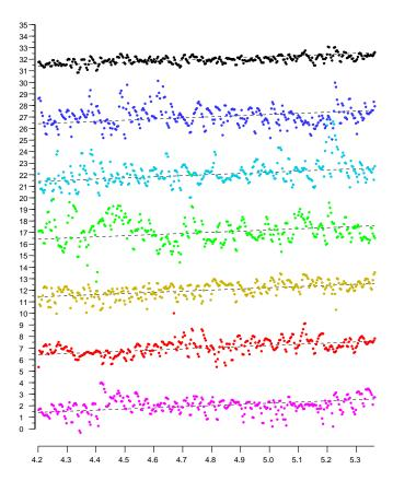
**Figure 6.** Sample plots (colored) of reported distances in six 80 MHz wide channels in the 5 GHz band. The top (black) plot is a simple average, which has less than half the error of the individual measurements. Horizontal axis: actual distance in meters. Vertical axis: reported distance in meters. (Note that the average slope of the plots is not equal to one, because the scales on the vertical axis and horizontal axes are different). (Individual plots are offset vertically to avoid overlap).
