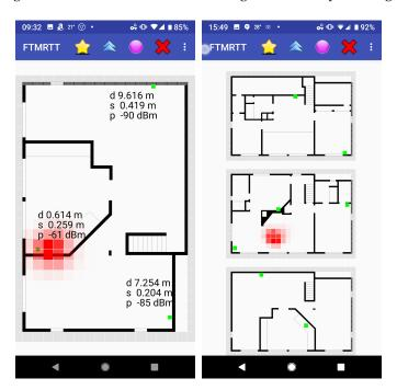
**Figure 11.** Sample "heat maps" of Bayesian grids. Left: 2-D case (single level) with 3 responders (green dots). Text shows current FTM RTT distance, st. dev. and signal strength. Right: 3-D case (three levels) with 7 responders. Voxels in each floor were collapsed into a single layer for display purposes.
