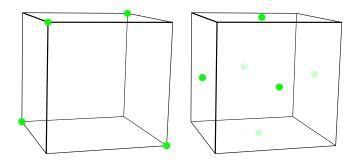
Figure A2. Left: Placement of 4 responders (3-D case) Right: Placement of 6 responders (3-D case).
