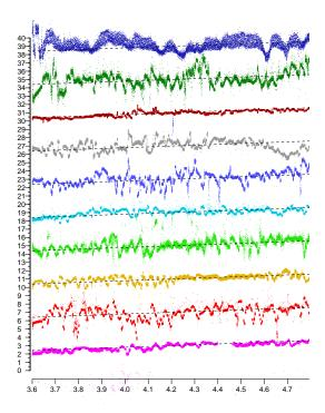
**Figure 3.** Sample measurements using ten responders in a range of positions (Top plot is for an access point operating in the 2.4 GHz band, the rest are in the 5 GHz band). Horizontal axis: actual position in meters. Vertical axis: reported distances in meters. (Note that the average slope of the plots is not equal to one, because the scales on the vertical axis and horizontal axes are different). (Individual plots are offset vertically to avoid overlap).
