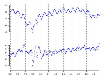
**Figure 5.** Upper plot: signal strength (RSS) in dBm, Lower plot: reported distance in meters. Horizontal axis: actual position in meters. Note undulations with wavelength somewhere between about half the wavelength and the full wavelength of the (2.4GHz) electromagnetic wave. (There is also an overall trend in RSS, probably due to destructive interference between the direct signal and a reflection off the concrete floor about 1.2 m below the line connecting the intiator to the responder).
