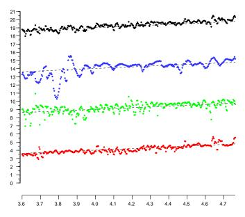
**Figure 7.** Sample plots (colored) of reported distances in three channels. The top (black) plot is a weighted average, which has only a bit over half of the average error in the individual plots. Horizontal axis: actual distance in meters. Vertical axis: reported distance in meters. (Note: the average slope of the plots is not equal to one, because the scales on the vertical axis and horizontal axes are different). (Individual plots are offset vertically to avoid overlap).
