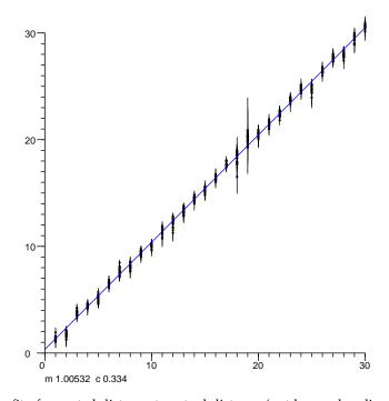
**Figure 4.** Linear fit of reported distance to actual distance (outdoors, clear line of sight (LOS), no obstructions in the first Fresnel zone). The offset in the well calibrated setup tested here happens to be small (less than half a meter), but can be five meters or more in other situations. Horizontal axis: actual position in meters. Vertical axis: fine time measurement (FTM) of the round trip time (RTT) reported distances in meters.
