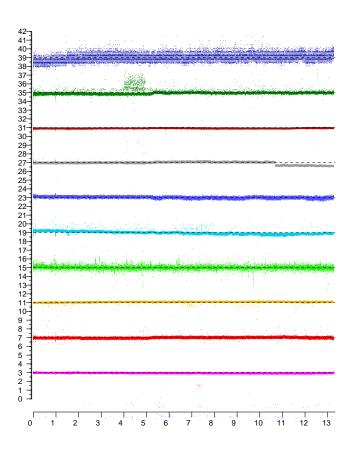
**Figure 2.** Sample measurements using ten different responders in fixed positions. (Top plot is for an access point operating in the 2.4 GHz band, the rest are in the 5 GHz band). Horizontal axis: time in hours. Vertical axis: distances in meters (individual plots are offset vertically to avoid overlap).
