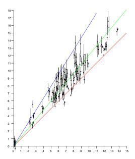
**Figure 8.** Scattergram of measured distances versus actual distance in wooden three-story house. Vertical axis: measured distance (meters). Horizontal axis: actual distance (meters). Red line (slope 1) is the ideal relationship; Green line (slope 1.2) is the best linear fit; Blue line (slope 1.6) is an upper extreme. The high permittivity of building materials biases the distances measured by FTM RTT.
