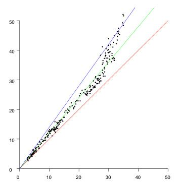
**Figure 9.** Scattergram of measured distances versus actual distance in a large open plan office building. Vertical axis: measured distance (meters). Horizontal axis: actual distance (meters). Red line (slope 1) is the ideal relationship. Green line (slope 1.2) is the best linear fit. Blue line (slope 1.4) is an upper extreme. The high permittivity of building materials biases the distances measured by FTM RTT.
