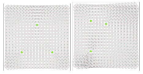
**Figure A1.** Quality of position determination near three responders (2-D case). Left: Symmetric arrangement. Right: Asymmetric arrangement.
