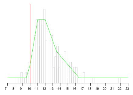
**Figure 10.** A slice through a particular observation model. Horizontal axis: measured distance (when actual distance is 10 m) Grey histogram: measurements from typical three-level residence. Green curve: observation model—probabilty of measuring the specified distance (piece-wise linear fit to grey histogram).
