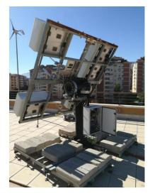
Figure 8. The designed high-concentration photovoltaic system (HCPV) tracker.
