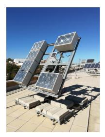
Figure 7. The designed high-concentration photovoltaic system (HCPV) tracker.
