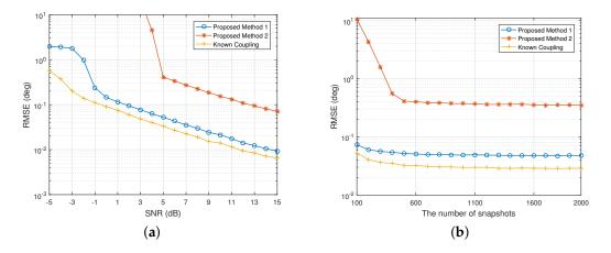
**Figure 1.** RMSE of the DOA estimates of 2 independent signals versus (a) SNR when N = 500; (b) *N* when SNR = 5 dB.
