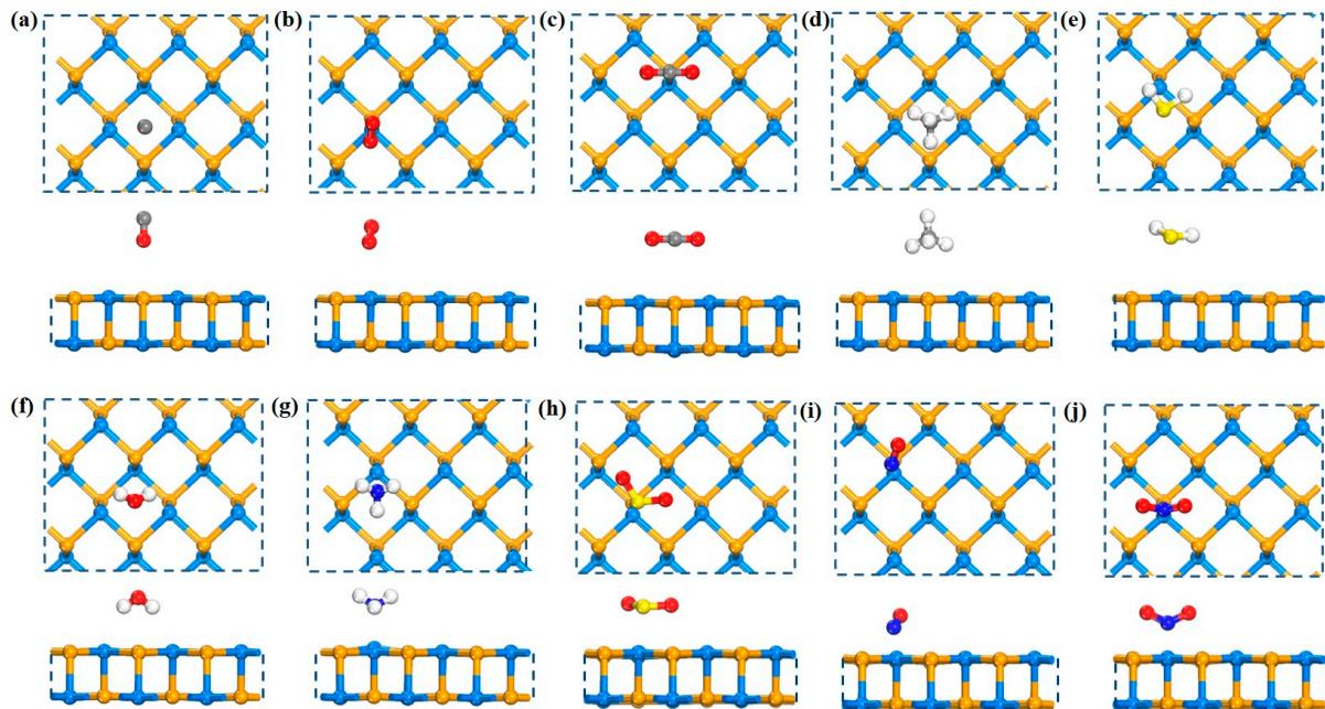
**Figure S2.** Front and top views of gas molecules adsorbed on a SiSe substrate. Gas in turn are CO, O<sub>2</sub>, CO<sub>2</sub>, CH<sub>4</sub>, H<sub>2</sub>S, H<sub>2</sub>O, NH<sub>3</sub>, SO<sub>2</sub>, NO and NO<sub>2</sub>.
