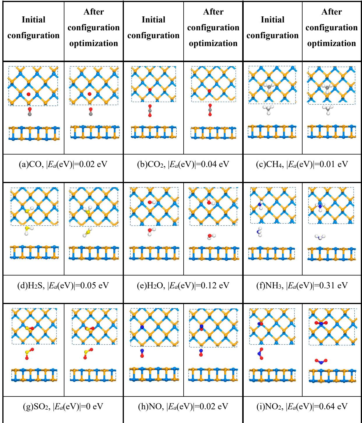
**Figure S1.** Front and top views of gas molecules adsorbed on a SiSe substrate in a different molecular orientation. Gas in turn are CO, CO<sub>2</sub>, CH<sub>4</sub>, H<sub>2</sub>S, H<sub>2</sub>O, NH<sub>3</sub>, SO<sub>2</sub>, NO and NO<sub>2</sub>.
