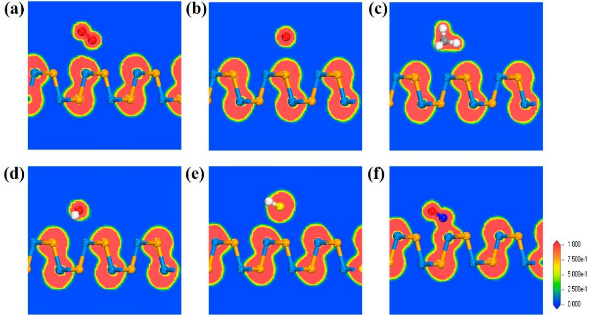
**Figure S4.** The distribution of electron localization maps of (a) O<sub>2</sub>, (b) CO<sub>2</sub>, (c) CH<sub>4</sub>, (d) H<sub>2</sub>O (e) H<sub>2</sub>S and (f) NO configurations. The reference column for the ELF value from 0 to 1 is located on the right side of the figure. The slice of the ELF is parallel to the (100) crystal plane.
