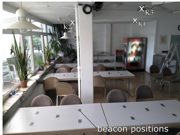
**Figure 19.** Experimental scenario for the machine learning experiments. A beacon is put on a table approximately at the marked cluster positions and the aim is to correctly estimate the cluster it is in by training each machine learning algorithm with the TDoA measurements of multiple positions on the tables.
