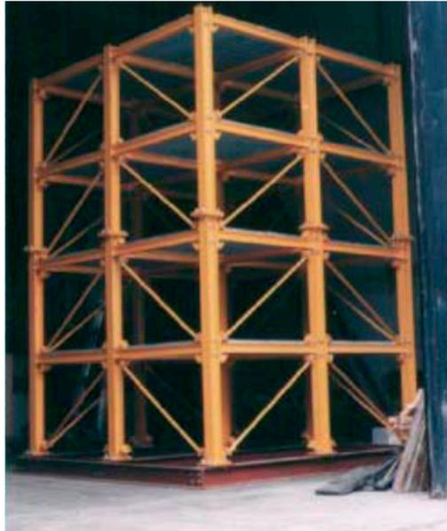
**Figure 3.** American Society of Civil Engineers (ASCE) structural health monitoring benchmark structure.
