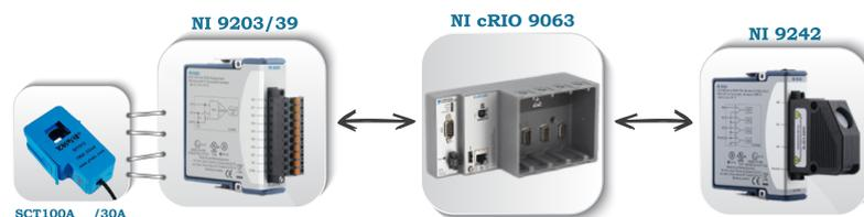
**Figure 3.** Basic components of IMPEC systems.
