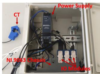
**Figure 2.** The IMPEC system with highlighted components in an enclosure box.
