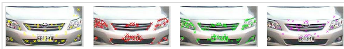
Figure 5. Detected feature points using KAZE, FAST, BRISK and SURF feature detectors respectively.
