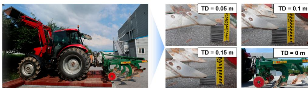
Figure 6. Soil non-penetration test of the real-time tillage depth measurement system.
