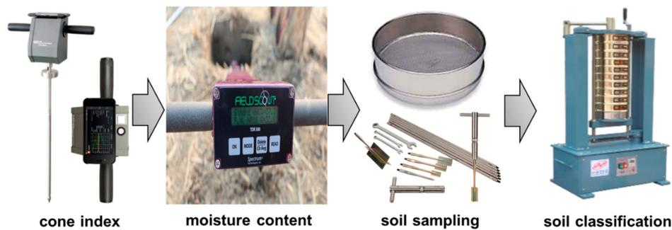
Figure 1. Measurement process of soil physical properties.
