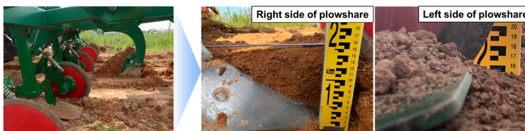
**Figure 9.** Manually measured tillage depth in test field.
