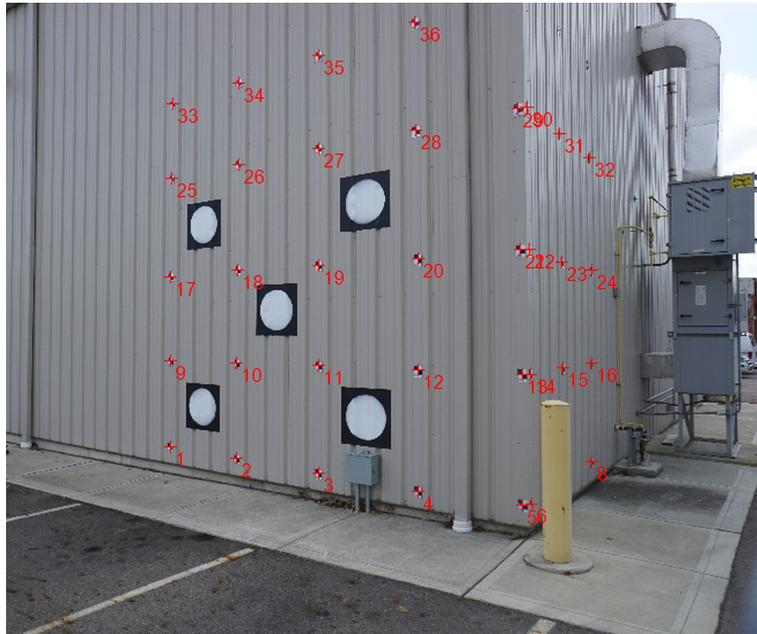
Figure 8. LiDAR targets.
