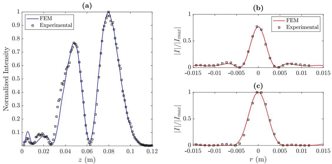
**Figure 7.** (a) Measured (black squares) and simulated (blue line) focusing profiles (longitudinal cuts) for the manufactured BiFZP lens. (b,c) Measured (black squares) and simulated (red lines) transversal cuts at  $z = F_1'$  (b) and  $z = F_2'$  (c).
