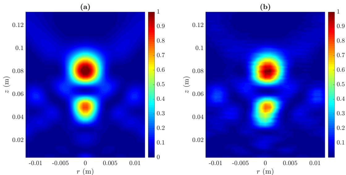
**Figure 6.** (a) Simulated and (b) measured normalized acoustic intensity maps for the manufactured BiFZP lens.
