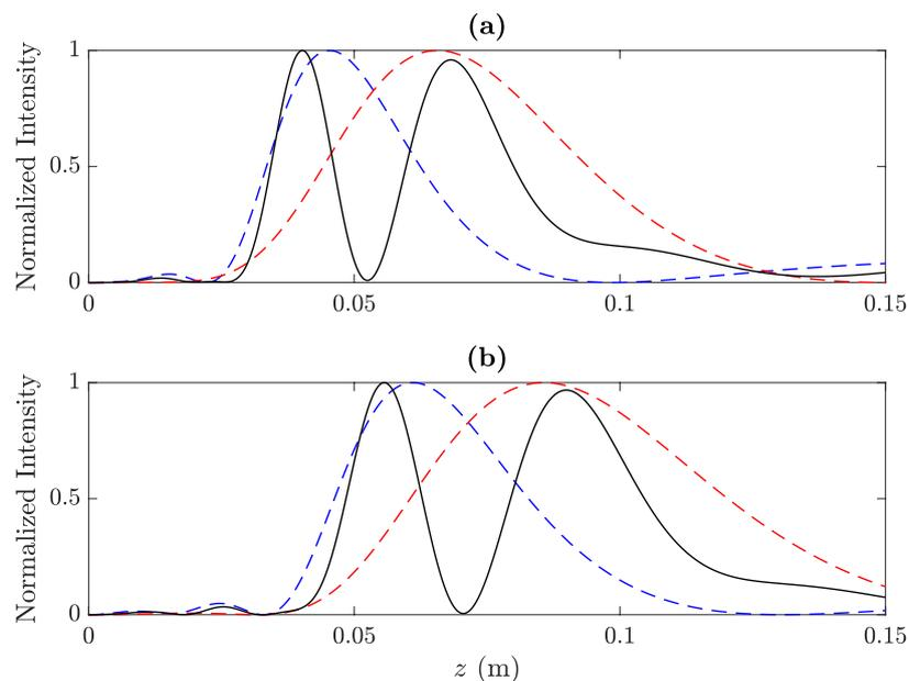
**Figure 3.** (a) The BiFZP focusing profile designed for  $F'_1 = 40$  mm and  $F'_2 = 68$  mm, and (b) the BiFZP focusing profile designed for  $F'_1 = 56$  mm and  $F'_2 = 90$  mm. In both cases,  $f_0 = 250$  kHz.
