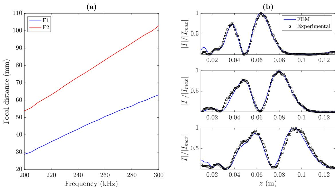
**Figure 8.** (a) BiFZP focal distance for  $F_1'$  (blue) and  $F_2'$  (red) as a function of the operating frequency and (b) BiFZP focusing profiles at 220 kHz (top), 250 kHz (middle) and 280 kHz (bottom).
