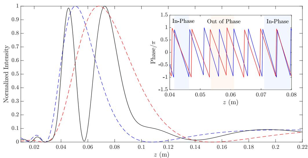
**Figure 2.** The bi-Fresnel zone plate focusing profile (black) compared to the inner (blue) and outer (red) focusing profiles. The phase of the inner (blue) and outer (red) profiles are shown in the inset.
