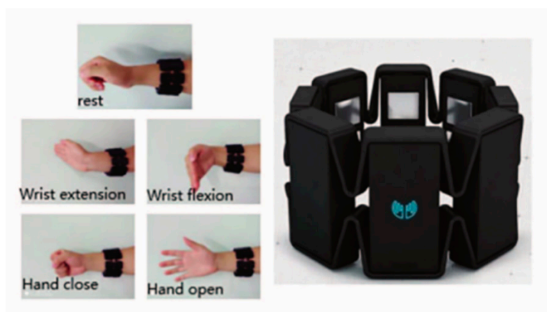
Figure 6. The 5 hand/wrist gestures and Myo armband. In this figure, the left is a schematic diagram of five gestures, and the right is the Myo armband.
